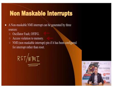
It can be generated because one of the oscillators, and you know that there are three oscillator sources in your MSP430 microcontroller if any of the oscillator is not working the way it should it can generate non-maskable interrupt.
