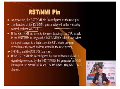
Here is details of, here are the details of the RST/NMI pin. At power-on, when you power up, when you turn the power on, the RST/NMI pin is configured as reset pin, and the function of the RST/NMI pin is selected in the watchdog control register.
