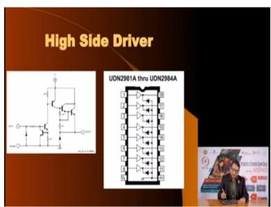
Similarly, for P and B, either you can use individual PNP transistors or you could also use this driver IC called UDN2981.
