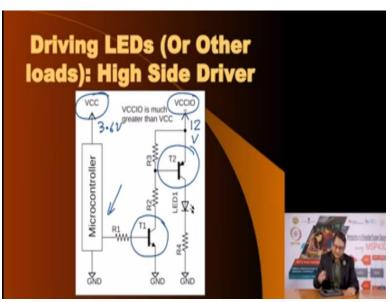
And this is the configuration that we require that instead of apart from the transistor T2 now, which is the PNP transistor, we also need another transistor T1, which will isolate the voltage that appears at the output pin and ensure that transistor T2 can be turned on or off. Let us understand the voltages that are available here.
