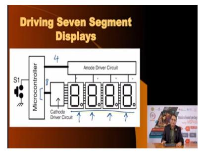
Let us see what it looks like. Here I have a configuration where we have 4 7 segment displays as I showed here. As we have seen earlier a 7-segment display requires 8 pins. So, if we want to control 4 7 segment displays, it would require that the microcontroller has 32 pins, but what if we do not have 32 pins. Can we control these 4 7 segments displays with less number of pins? It turns out yes using this configuration.
