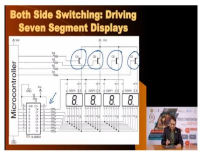
For such a configuration here, I have created a schematic for you which shows 4 7 segment displays common anode type and as you see here, we have 4 PNP transistors and instead of individual 8 NPN transistor we have used a IC which consists of 8 NPN transistors that IC is a low side driver.
