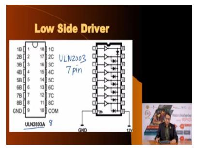
This is the IC. In the electronic components that we expect you to have, you may recall that we have an IC called ULN2003. It is exactly like 2803 except ULN2803 has 8 control pins, but ULN2003 has 7 pins that is you can control 7 switches.
