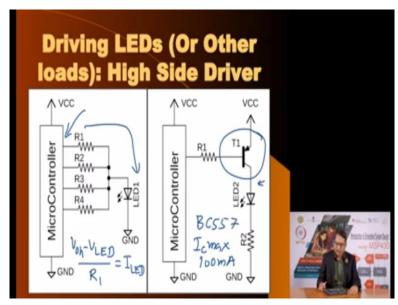
This is the high side switch and this is the way to calculate the value of the base resistor. We already seen the value, the way to calculate the value of the series resistance. Let us see what other configurations we have.
