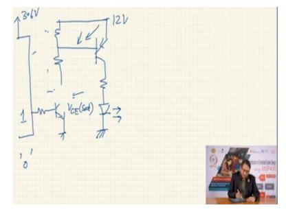
Now, we have a PNP transistor where the VCC is 12 volts. Here is our load through the resistor and LED and we have now registered driving a npn transistor and at the base of the resistor, we have created a voltage divider. This is connected to 12 volts. This has a supply voltage of 3.6 volts. Now, when I output logic 1, this transistor will be saturated and therefore the voltage here will be close to, this will be VCE SAT, which is a very low value say 0.2 volts.
