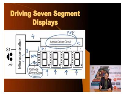
So, this is a very effective method of controlling large number of displays using less number of pins, but at the cost of additional circuitry. In this case what we call as anode driver circuit, and
