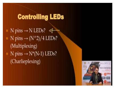
Now, we have to consider the situation like we considered for the switch case that when you want to connect a few number of switches, you can 1 switch each to each pin. As the number of switches increase, you have to optimize the number of pins by creating a matrix and if you have N pins output and N pins input that is total number of 2 N pins, you are able to control n square switches. In the same configuration, how about if we want to control large number of LEDs.
