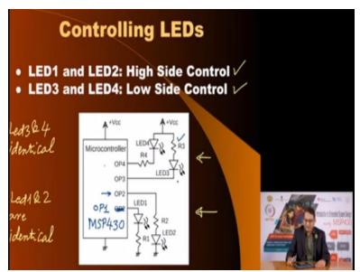
Now, here we see we have the VCC here. Now, if the VCC itself is 3 volts then it may be difficult to control a blue LED but MSP430 can, the supply voltage can go up to 3.6 volts. So, we can power this with say 3.6 volts and we will be able to connect blue LEDs also. However, in the calculations we must use a forward voltage drop across an LED appropriately so that we can estimate the value of the resistors.
