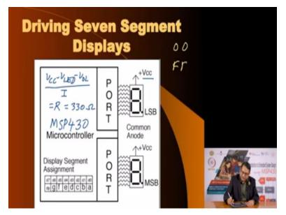
The second method would be to use common anode LEDs. Now, here the anodes are common. Therefore, it is connected to VCC and the cathodes are the segments which is a b up to dp. They are connected to port pins. This is your MSP430 microcontroller and here the calculations will be same as we saw. This is low side control and so the calculations would be what we did is equal to the resistor value will be to VCC minus VLED minus VOL divided by the current that you require.
