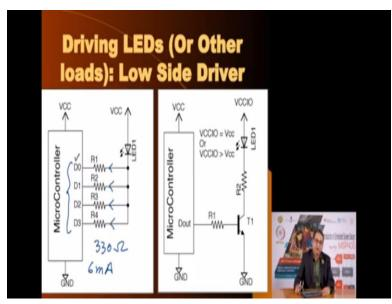
Now, here is what I meant when I mentioned that what if you wanted to increase the intensity of the LED. Now, each of the port pins of the microcontroller has only a limited amount of capability. As we have seen for MSP430, the maximum current that each of the pins can provide
