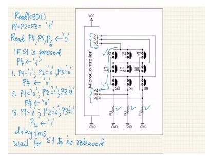
So, this Read keyboard function let me describe it here with call this subroutine as Read KBD, short for Read keyboard. This function will be called by the microcontroller and it will perform the task of identifying if any switch has been pressed and if a switch has been pressed, what is the code of that switch?
