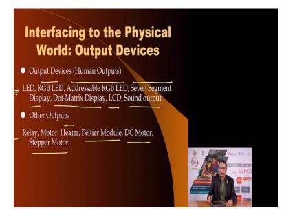
Now, let us see how we can connect some output devices to our microcontroller system and these would form from the, the output box and we see the ways multiple ways in which microcontroller can interact with the outside world would be through LEDs of various types. As we had listed in that block you have LEDs, normal LEDs, you have RGB LEDs. You can also addressable RGB LEDs, you have 7 segment displays.
