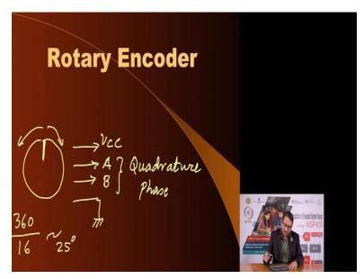
But electrically it has 4 pins. One of the pins is VCC that means you have to connect it to VCC. Another is ground and there are usually two outputs labeled A and B. What it does is let us say this is the reference point of this Rotary Encoder, as you move it either clockwise or anti clockwise, it would give you pulses on A and B outputs. And the rate of the pulses that you are getting will indicate that you are moving the Rotary Encoder fast.
