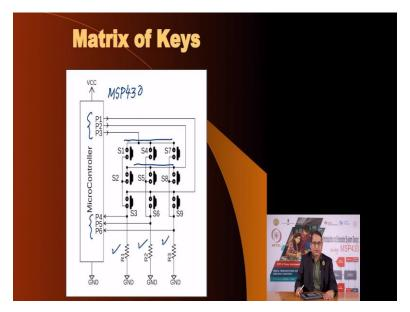
This is the matrix of Matrix of Keys. Here we see the microcontroller we have is a MSP430 let us say it MSP430 and 3 of these pins P1, P2, P3 will be programmed as output. The other 3 pins here P4, P5 and P6 will be programmed as input. And we see that P3 is connected to these 3 switches S1, S4 and S7 to one end of these 3 switches, P2 is connected to S2, S5 and S8 here and P1 is connected to S3 S6 and S9.
