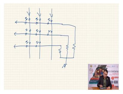
One, the argument behind the matrix is as follows that you would create row and column let us say, I create a row and column of 3 rows and three columns. And I connect 3 registers, which are pull down resistors and these are going to come to columns are going to come from output pins of microcontroller.
