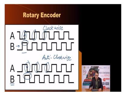
So, I have drawn the two sets of pulses, these are the output on A and B in one case this could be, this could be clockwise motion of the encoder may give you this relationship between A and B as you see, if you consider the reference to be B, that means during the time that B is high, A is going from 0 to 1.
