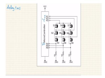
Then what it will do it is going to again, when the switch is released again the switch debounces, switch bounces and so it must debounce it so it is going to again called a delay sub routine of 1 millisecond.
