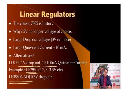
Instead, people are using low dropout voltage regulators. And I already mentioned the characteristics that they offer. A low voltage of 0.1 volt drop out and about 10 to 100 micro amperes of quiescent current. Here are some examples. If you want to power a 5 volt or a 3 volt or a 2.7 volt circuit, you can use LP2950 this comes in various versions which provide 2.7 or 3 or 3.3 even 5 volt output another adjustable voltage regulator of the LDO variety is LP38500.
