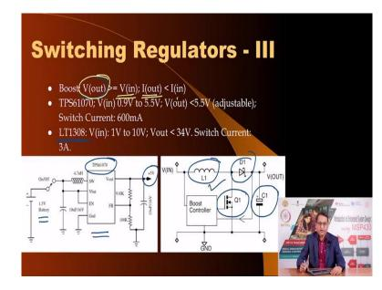
In case you need the output voltage to be more than the input voltage, then use a boost type of voltage regulator where the output voltage, as you see here, is more than the input voltage, but then the output current is less than the input current because at the end of the day, power has to be conserved.
