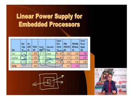
In the next slide I have taken from the data sheet of a high end Texas Instruments microcontroller. And as you see, it requires three power supply voltages 1.1 volts, 1.8 volts and 3.3 volts and you see the current expected out of these three power rails is such that the product is more or less uniform, so that when I have if I have this, IC usually it will be split in three parts, the periphery, the middle part and the core.
