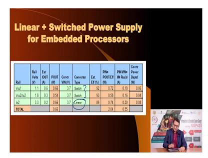
And so an ideal solution would be one in which the two, these two power supply's regulators are replaced with switching regulator and the third one is still maintain at of a linear type. This is the expectation out of a designer when you are designing a complete embedded system, you have to consider the power supply requirements of the microcontroller and other components in your system and to design voltage regulators compatible with the requirements.
