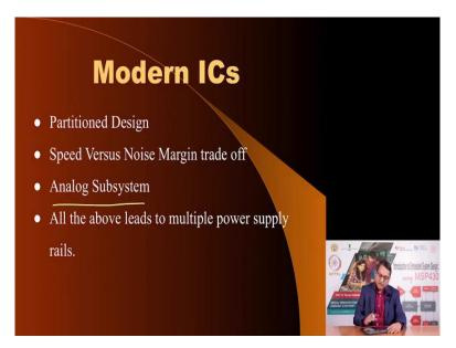
Modern ICs are designed such that the chip is partitioned in several parts the periphery of the IC often is operated at higher voltages and the inner parts are operated at higher frequency and therefore lower voltages so has to maintain a uniform power dissipation across the chip so as to maintain a uniform participation.
