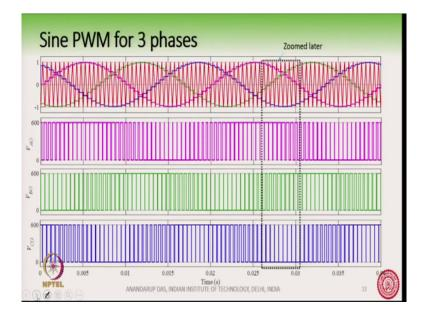
So, here on this diagram, we are showing the sine PWM, where you can see the high frequency carrier here and three sine waves three modulating sine waves balanced that corresponds to v A v Band v C. And then, we also have shown the pole voltages v AO v BO and v CO which is which are fluctuating between 0 and 600 Volt; the DC bus being 600 Volts. Now, let us zoom into this portion of the waveform. Let us zoom in here and show it in the next screen.
