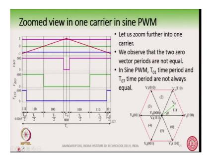
Then, there. So, this is that carrier. This is the carrier there and you have the three modulating wave forms; A phase, B phase and C phase here.
