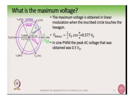
The maximum voltage can be obtained by observing the space vector diagram and the resultant vector which is inside this space vector diagram.
