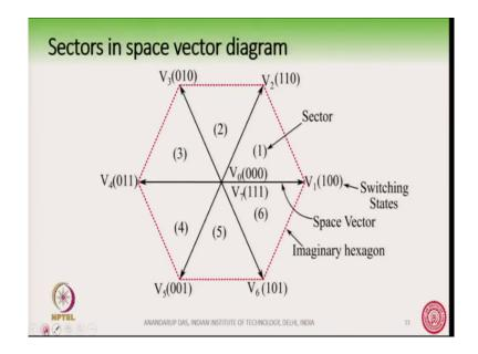
So, once we have made this boundary, once we have drawn this boundary, we can now divide the whole hexagon into 6 sectors ok. These sectors are 1, 2, 3, 4, 5, 6 as you can see in this diagram. The sectors are triangular in nature the reference vector at any point here can be realized by switching the three nearest vectors in the same sector where the reference vector lies ok. This we have seen now what is the maximum voltage?
