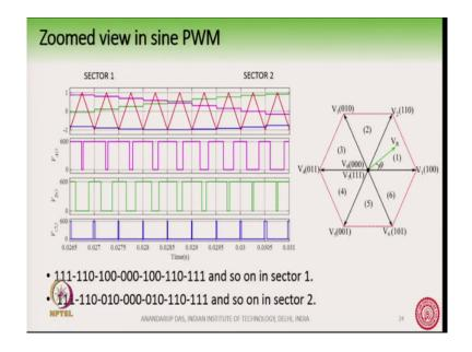
Let us concentrate here. Let us concentrate first in the first carrier that is we are first seeing here. How do you see the pattern of switching? The carrier is here and we are following the logic that if the modulating or the reference wave is more than the triangular wave, then we make the switch upper switch on so that we get the full DC bus voltage. When the modulating wave is less than the triangular wave, then the lower switch is turned on and we get 0 voltage.
