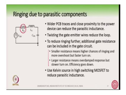
So, how can you mitigate it? Of course, if you use a wider PCB trace and close proximity to the power device you can reduce, you can reduce the parasitic inductance people sometime use twisted gate emitter wires rounding the loop. Now another way because since this is an under damped system another way to mitigate this effect is to put additional gate resistance ok.
