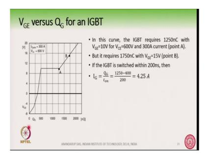
So, here this is a more specific example, which is again taken from the same datasheet of the device which we talked earlier and here you can see the values given right. So, this is the whole turn on process, you will see this turn on process starting from so, in this case the device was started from minus 8 volt.
