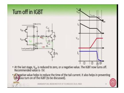
And then the ultimately at the fourth stage this voltage V G E goes to minus 5 volt and the IGBT will turn off fully ok. Another particular exam help why V G E is negative is that in case of IGBT there is a long tail current because there are excess minority carriers which needs to be recombined and so, in order to reduce or in order to, in order to quickly take away these minority carriers.
