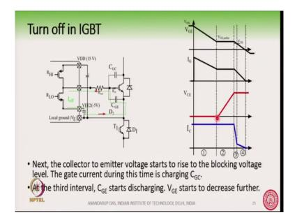
And then like the previous phase second stage V CE voltage is rising whereas, the current is still maintained and at the third interval the C GE starts decreasing that is this C GE capacitor is starting to decrease.
