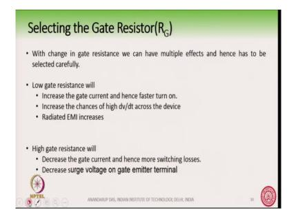
So, we see that the gate resister RG has, have multiple effects and it has to be selected very carefully. So, far we have only seen that suppose if you have a low gate resistance then, we can increase the gate current of course, if the resistance is low we can allow more current to flow and we can have a faster turn.
