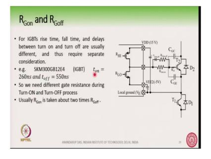
For example for this IGBT t on is 260 nanosecond and t off is 550 nanoseconds something like that ok.
