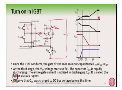
Now, what happens in stage the once the IGBT has started to conduct the gate driver, this gate driver is seeing a input capacitance which is the parallel combination of two of these
