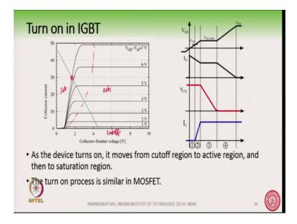
So, we can say that, if we see this I C versus V CE characteristics of the device then I can see that it has now moved from the cutoff region through the active region and have settled at the saturation region.
