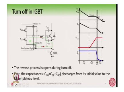
Now, the turn off process, that is the other process of course, the turn of process is an exact replica, but in a reverse fashion this just reverse thing is happening. So, at first the capacitances these two capacitances are discharging from their initial value. So, how is that? How is the circuit behaving? So, you can see here that this capacitance is going to be so, going to be discharge through this MOSFET during turn off, we will turn on this MOSFET and turn off this MOSFET.
