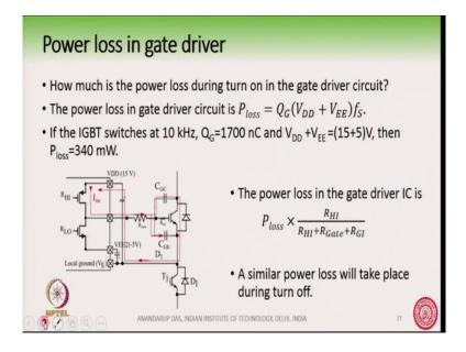
Now, what is the power loss in the gate driver as well as in the gate resistance? How much is the power loss? So, the because why this is important because not only we have to when we are taking a gate driver I C, we have to see how much current it can deliver and how much is the power loss that it can sustain to drive this IGBT ok.
