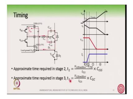
Again, approximate time how much is required in stage 2, again these are very crude approximations as I told you these values of capacitance and all they are varying with voltage. So, a very rough approximation is saying like the time required in stage 2 is how much the total charge. So, I G 2 into t 2 is the total charge and this total charge is equal to C times V so, V G E miller minus V threshold into C ISS.
