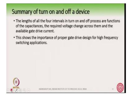
So, this is what I wanted to summarize that this length of all these four intervals in turn on and turn off process are function of the capacitors, the required voltage change across them and the available gate drive current ok. So, a gate drive design for high switching frequency application. So, it is important to properly choose these components. (Refer Slide Time: 42:31)
