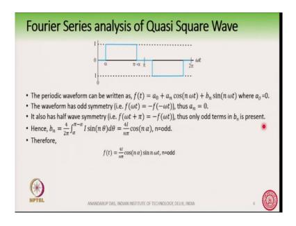
So, before going that, so let us analyse quickly, what are the harmonics present in this waveform ok. So, that we can at least know what are the harmonics that are getting injected into the supply. So, this is the periodic waveform and so, if you write the Fourier series, this is very standard notations.
