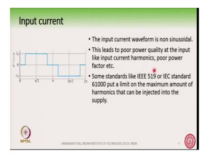
It has a lot of harmonics present in it. Now, the input supply voltage is sinusoidal. Typically, we can assume that the input supply voltage is almost close to a perfect sine wave. Now the input current drawn by this 6 pulse rectifier as you can see here is not at all sinusoidal ok, it is a quasi squared wave. Now this leads to poor power quality at the input. So, we are basically injecting a lot of harmonics into the supply ok.
