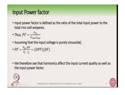
So, the input power factor is defined as the ratio of the total input power to the total rms volt ampere ok. So, the power factor is P in divided by V rms into I rms. Now, v rms is same as V in v 1, so P in by V 1. So, I can substitute P in by V 1 and what is I rms is distortion factor divided by I 1 from the definition of distortion factor.
