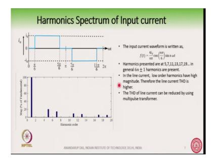
So, we see that we have all the odd harmonics present here ok. So, in this case, in the case of a, in the case of the input current drawn from the 6 pulse rectifier; the value of alpha is equal to pi by 6 as you can see here. So, if you put f t there cos n alpha so, you put n pi by 6 and then if you put the values of n as 3, 5, 7, 11 like that we find that all these fifth seventh
