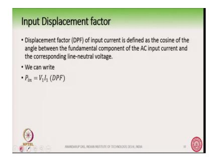
And, there is also one more definition that is called the input displacement factor. So, the displacement factor of the input current is defined as the cosine of the angle between the fundamental component of AC current and the fundamental AC voltage ok. So, fundamental AC voltage and fundamental current the angle between them cosine of that angle is called DPF or Distortion Power Factor ok. So, the power input is V 1 I 1 into distortion power factor.
