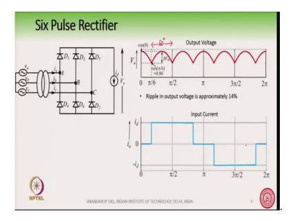
Now, if you see so, this is the six pulse rectifier ok. So, here you can see we have a input AC and we have a transformer and then, the transformer is fed through a 6 diode bridge rectifier, three phase diode bridge rectifier and on this side we have a current source which is acting or which is representing the load ok. Now usually, we have the transformer here.
