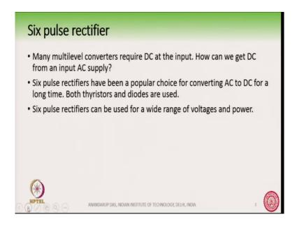
Now, many multi level converters, not only multi level converters, but many normal conventional two level VSI or VSC, they have the DC at the input ok. So, the DC bus is present on in such voltage source converters. Now the question is how do we get that DC? We get that DC from an input AC supply right. Of course, we can also get the DC from a battery or from other steep DC sources. But in many of the multi level converters, we get the DC by rectifying the input AC supply.
