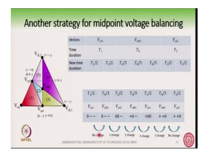
Next, how am I going to apply the vectors? So, we will now place these timings in a different fashion, not in this sequence ok. So, you see how we are going to place the timings first. So, this T 1 by 2 comes here, but then I have a T 0 by 3 time which I go from here to here.
