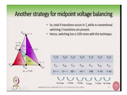
However, if the switching frequency is sufficiently high which is most of the case in applicable, then this poorer harmonic performance may be acceptable it should not be any problem because if the fs or because in this case the harmonics will recited 2 fs. So, in that 2 fs we can filter it out the harmonics.
