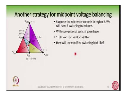
Now, one question that will automatically come up now in your mind is that; this V zM 1 is a combination of 3 vectors ok. V zM 1 is not a vector which is obtained from a direct switching. V zM 1 is obtained by switching of one third of these 3 vectors here. So, will it not increase the switching frequency? Yes, indeed it will be increasing the switching frequency and that is correct.
