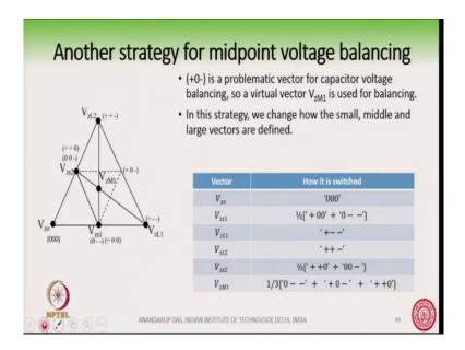
So, remember that we had said that plus 0 minus or the medium vector or the middle vector was the problematic vector ok, for the capacitor voltage balancing. So, this vector plus 0 minus, this vector will not be directly used ok. And we will redefine how we define the vectors in the sector. So, that is why you see here we have not so, we have used these black circles for the vectors, but we have not used any black circle here.
