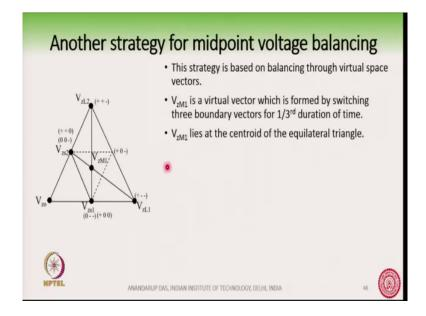
But for different durations of time for example, this vector one example say of a virtual space vector is V zM 1 ok. So, this is the vector here. This vector does not exist because, we do not have any switching state which will produce this vector. Of course, we have switching states that produce this vector, this vector, this vector, this vector and this vector. So,
