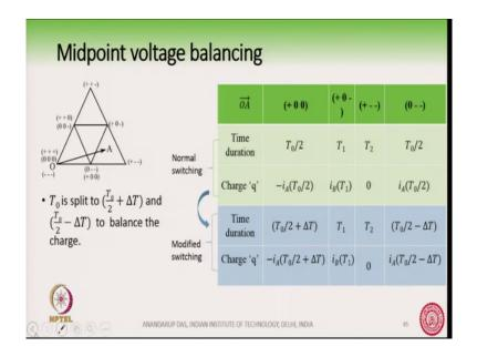
So, this is shown in the next cycle next table here ok, but first we I would like to say that. So, this means that what we are doing here is T 0 by 2 and T 0 by 2 instead of having equal T 0 by 2, we will make these two these two multiplicities or these two switching multiplicities to be not equal to T 0 by 2, something other than T 0 by 2. So, that the effect from i B into T 1, the net charge which we can make it we will try to cancel the effect of i B into T 1.
