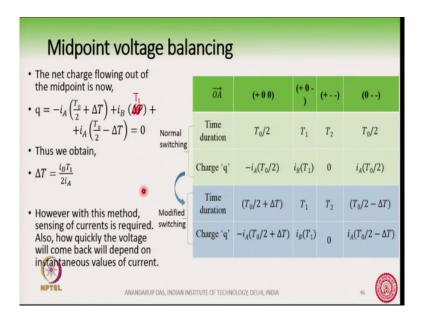
So, now we can equate. So, what we can equate? The net charge flowing out of the midpoint q is minus i A, T 0 by 2 plus delta. This is for the plus 0 0 duration here. For the plus 0 minus duration, we have i B into delta T this one coming.
