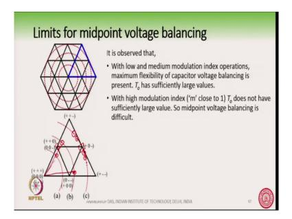
There is also one more limitation of this technique. And this can be understood from this space vector diagram. So, here you see that so, this is the space overall space vector diagram and I am drawing the 3 reference vectors means for different modulation index. So, this is like a for small modulation index, this is for medium modulation index and this is for large modulation index; the 3 reference vectors ok.
