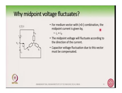
What will happen with the medium vectors ok. So, let us take this plus 0 minus combination the medium vector which is this one on the space vector diagram this one this is the medium vector so, plus 0 minus. So, what is its effect on the midpoint voltage.
