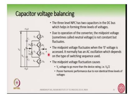
So, this is a topic. So, first we will understand why the midpoint voltage of the NPC fluctuates during the operation of the converter. First we will understand and subsequently we will see two techniques of mitigating this issue. So, the first technique will be kind of, the second technique is a superior technique to the first one and we will see how this works these two techniques work.
