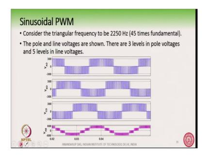
So, suppose if the triangular frequency is 2250 Hertz that is 45 times the fundamental where the fundamental frequency is taken as 50 Hertz ok. So, here we see the pole voltage and the line voltage waveforms based on the logic which we had just described in the last slide ok.
