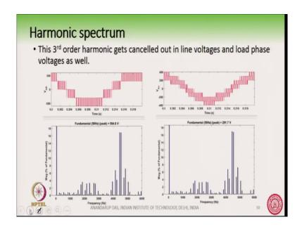
Of course since this is 45, I mean this is a multiple of 3 and we know that in the line voltage this third harmonic component will disappear ok. So, we will in the; so this is the line voltage waveform and this is the load phase voltage waveform and you can see that the 2250 that is a 45 th one has disappeared.
