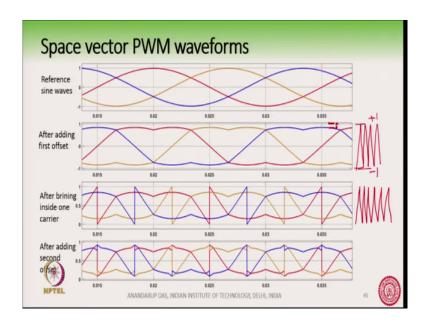
So, first let us start with this reference sine waves this is a sine wave as you can see here 3 sine wave references here we give the first offset. So, what we did in like a conventional voltage source converter after adding the first offset which is nothing, but this V max and V min divided by 2.
