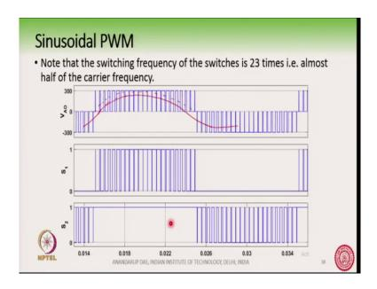
Now, here this waveform shows the V Ao voltage as well as the upper 2 switches S 1 and S 2 the pulse pattern given to this the gate pulse for S 1 and S 2 are given here ok. Now, in this case you see there is a change of pattern of the 2 switches S 1 and S 2, first let us observe how many times S 1 is switching in a cycle.
