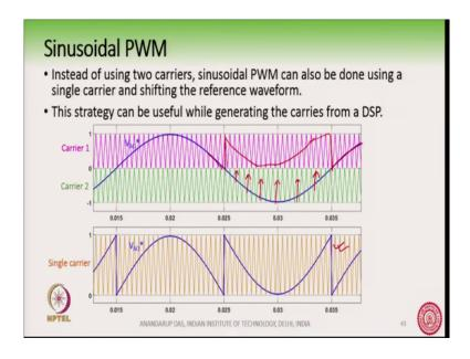
So, this is the drawback of sinusoidal PWM. So, before I go into space vector PWM before I would say that instead of using 2 carriers it is possible to use a single carrier also ok. So, you can see here there are 2 carriers, but you can also have a single carrier right. So, it is useful while generating the carriers from a DSP; because then we will need 1 carrier from the DSP.
