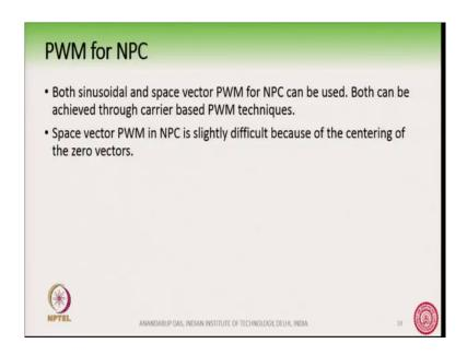
So, we look into now into the PWM or Pulse Width Modulation strategies for neutral point clamped converter specifically 3 level NPC. Now, for switching NPC we can use both sinusoidal as well as space vector PWM can be used both of them; and both of them can be achieved through carrier based PWM techniques ok. And in this case the space vector PWM
