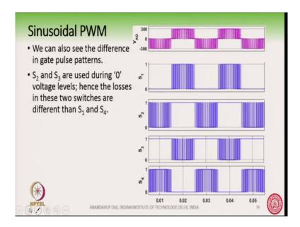
So, we can also see it here in this diagram. So, we can see therefore, that in NPC the uneven loss distribution in the switches is a challenge and for which we have other topologies where the loss distribution has been specially taken care of.
