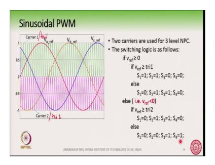
So, this is what we will see now. So, at first we will see the sinusoidal PWM strategy we will see the sinusoidal PWM strategy and then we will see the space vector PWM strategy. Now in sinusoidal PWM strategy for a 3 level NPC we see that we have a sinusoidal or we have 3 sets of sinusoidal modulating wave forms and carriers ok.
