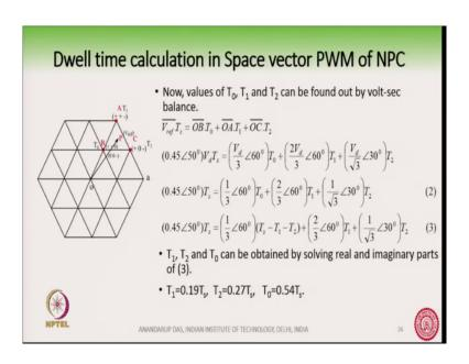
Where we had talked about that T 1, T 2 and T this slide you can refer to this slide and can find out how we can calculate the timings for the 3 nearest vectors. As you can see this requires a lot of calculations this requires a lot of calculations and this can be simplified much by using carrier based PWM technique ok.
