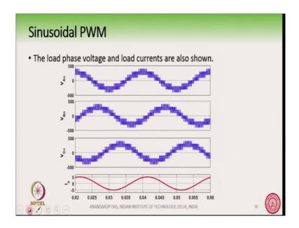
And the load phase voltage and the load currents are as shown here ok. So, this is the load current we had taken a I means an inductive RL load with a power factor close to unity like 0.9 or something close to that ok.
