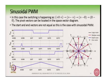
So, you can see that what is I have written the pivot vectors can be located in the space vector diagram. So, these so, you will see that the switching and the starting and ending vectors are all starting from this 6 pivot vectors; however, one thing that we must observe here is that the starting and ending vectors are not equal ok.
