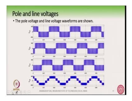
So, after we have done this. So, we can see the pole voltage and line voltage now we are in the space vector PWM. So, we have ensured that we will see this now we will ensure that the start and end vectors in a cycle in a switching cycle Ts will be of equal duration of time that is how space vector PWM is ensured right. So, here you see the pole voltage and line voltages. So, these are the pole voltages these are the line voltages you cannot differentiate much from sine PWM.
