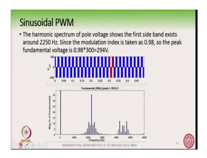
Now, if you do the harmonic analysis of the whole voltage. So, it shows that you see here the first band of harmonics reside around this 2250 Hertz ok. Which is 45 times the fundamental and this is what is expected ok. So, the harmonics are residing around the carrier frequency. Whereas, the second band exists around 4500 Hertz and third band will reside around 6750 Hertz and so on ok.
