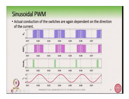
Now, again further if we go deep if we go one step inside the converter we can even see that for example, the actual conduction of the switches exactly which will be again dependent on the direction of the current ok.
