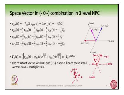
So for example, there is also one more example we have given here. So, suppose v AO t is for example, this is minus 0 minus combination, ok. Minus 0 minus combination, so, you put v AO t minus V d by 2 v BO t 0 and v CO t also minus V d by 2 and then you can find out v An t again like this. And then V R t are the resultant space vector as one-third V d e to the power j 2 pi by 3.
