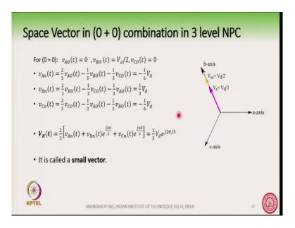
So, plus means the A phase is at V d by 2 and minus means the if B-phase is at minus V d by 2 and minus again means another minus means C-phase is at minus V d by 2. So, you can have 3 possibilities here, plus minus or 0, ok. On the A-phase, plus minus and 0. Similarly, you can have plus minus and 0 on the B-phase and plus minus 0 on the C-phase thereby, you have 3 into 3 into 3 that is, 27 possibilities. And which are listed in the table.
