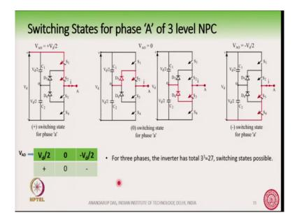
So, first we will see that in case of a 3-level neutral point clamped converter, the pole voltage has 3 switching states or 3 possibilities of the voltage not 3 switching states the pole voltage has 3 possible levels of output voltage. So, it can be V d by 2, it can be 0 or minus V d by 2. These are the 3 possible voltage levels that is at the point A with respect to the point o, so here.
