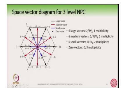
So, that forms the whole space vector diagram which is now shown in this figure, ok. So, these this is the whole space vector diagram. Again, sometimes so, these vectors are shown by these arrows. So, there are 6 here and there are like 12 large vectors sorry 6 large vectors and 6 medium vectors. So, the small vectors are given are indicated by the blue arrows while the medium vector is indicated by the red arrow and the black one indicates the large vector.
