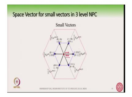
So, let us see that with these combinations how we get the vectors? So, these 6, so, there are the overall space vector diagram has 2 hexagons, the inner hexagon can be obtained by these switching state combinations which have been shown in the diagram, ok. So, if you take these combinations here, then you will always get to these 6 vectors on the inner hexagon, ok.
