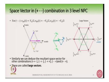
So, again I will so, this is shown in this space vector diagram, this will form the boundary of the space vector diagram. So again, I will use the dotted line to show you the inner hexagon, here and you have the outer, the vertices of this hexagon these are called the large vectors. And these are typically these are typically formed with switching state combination with like 1 vector as plus or 1 or 2 vectors as plus and the other vector as minus like that, ok.
