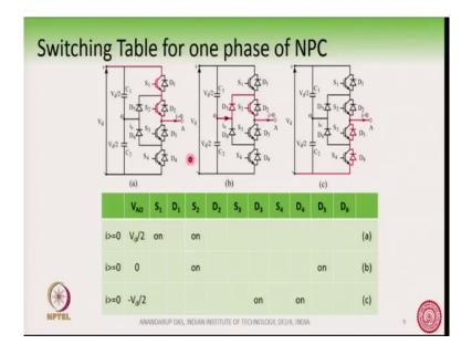
Give pulses to S 1 and S 2 ok, means; comparing this figure with along with this figure, I can say that if I want to get V AO voltage to be equal to V d by 2 then give positive gate pulses to S 1 and S 2 ok. Do not give pulses to other switches. If the current direction is positive, then S 1 and S 2 will flow will conduct where as if current direction is negative then D 1 and D 2 will conduct.
