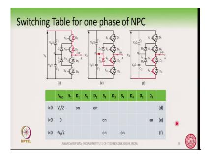
Now, when I is flowing into the converter like we have shown. Suppose, we want to get V d by 2 voltage. So, we would like to have so, what is our aim here? We would like to have V d by 2 0 and minus V d by 2 these three levels of voltages between point A and O. This is what we design and the current through point O should be bidirectional in nature. It is an AC current ok. It can be going out to the a terminal or it can flow inside the a terminal.
