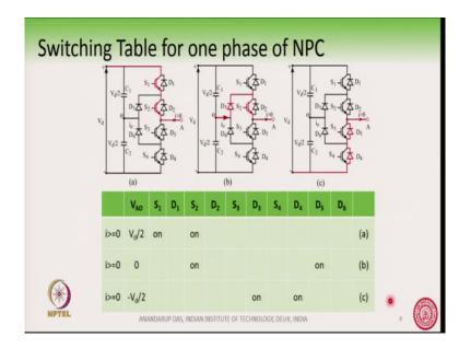
So, we have taken here one phase. So, first of all let me clarify this is a DC bus voltage which actually is split into two parts using this capacitor ok. So, the midpoint of this two capacitor is what is being accessed by the converter. So, there are no two separate DC sources, but the dc source is split into two parts using two capacitors and the midpoint.
