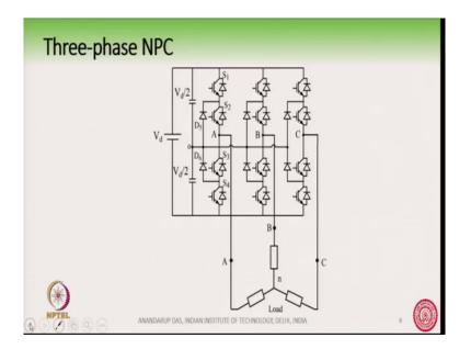
So, this is the three phase NPC circuit and let us now understand the operation of this circuit in details. In order to understand the operation of the circuit in details, we take only one phase of the converter and analyze it in details. So that, we can also understand the other phases, other phases are identical in operation. (Refer Slide Time: 00:35)
