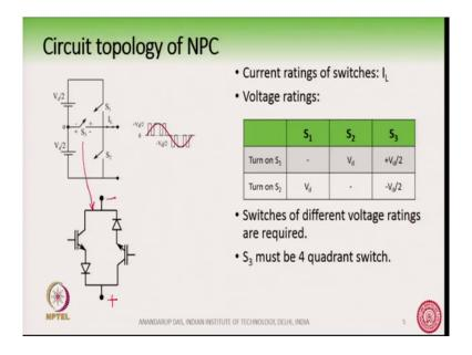
Now on the other hand if you have a situation like this, then once you turn on this transistor the current will flow like this; this is a bi-directional voltage, this circuit can block bi-directional voltage. So, we need S 3 as something like this here; S 3 must be made something like this, this kind of a circuit here.
