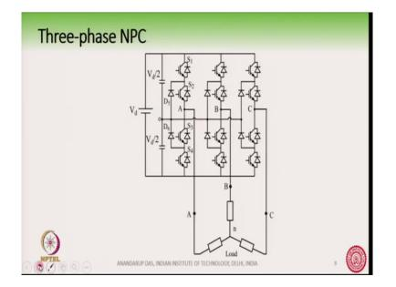
Here you see that, you have this as the one phase, the midpoint of the capacitor is connected to this point here; it is also connected here for the B phase, it is also connected to here at the C phase.
