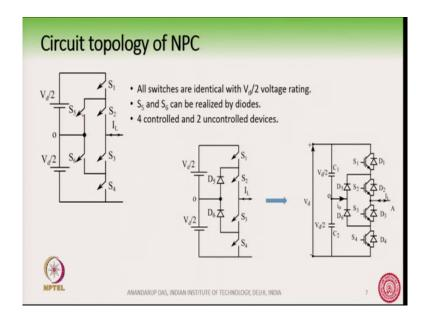
So, then if you explain this a little bit, but S 5 and S 6 may not be IGBT and anti parallel diodes together or a transistor anti parallel diode together, it is not needed. So, we can only have diodes here D 5 and D 6.
