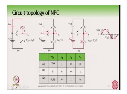
So, let us now see that if I use such a circuit, how can I get three levels of waveform output, ok. So, if I turn on suppose I, this is shown in this figure and also in this table. If I turn on S 1 here and I turn off S 2 and S 3 down on S 1 and I have turned on S turned off S 2 and S 3, I have turned on S 1; then the I get with respect to this O point or 0 point V A O, I will say O point the voltage V A O is V d by 2.
