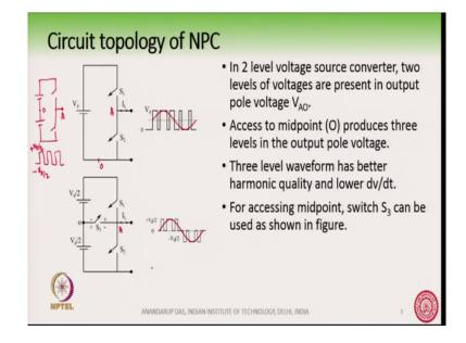
Let us first start with how did we obtain the NPC? So, when this transistor based voltage source converters became popular, people were using the two level VSI or two level voltage source converter. And typically they were using two switches like this here, it is still used. So, it is the most frequently used voltage source converter two switches like this.
