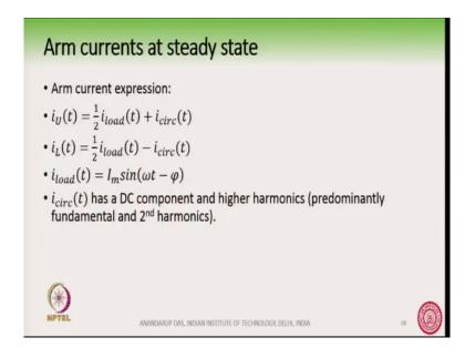
So, in the last class we had covered up to the point where, we said that there is a arm current at steady state which has both DC component as well as an AC component.
