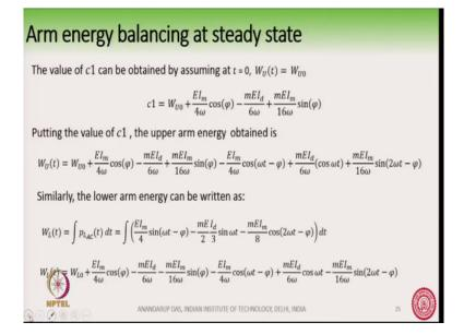
So, we take a integration constant c 1 and then we, the value of c one can be obtained by assuming that at t equal to 0, the initial arm energy is W U 0. So, then you can substitute and
