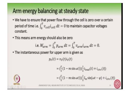
And we said that in order to maintain the capacitor voltage is constant, the DC component. So, we found out the instantaneous power for the upper arm and the lower arm. And we said that the instantaneous power the DC and the AC component should match ok. (Refer Slide Time: 01:28)
