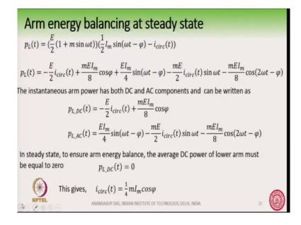
But, in the last class we also said that there is a there is an AC component of the power expression and this AC component for example, for the lower arm is like this. This is the AC component of the lower arm power. And similarly, there will be an AC component of the upper arm instantaneous power.
