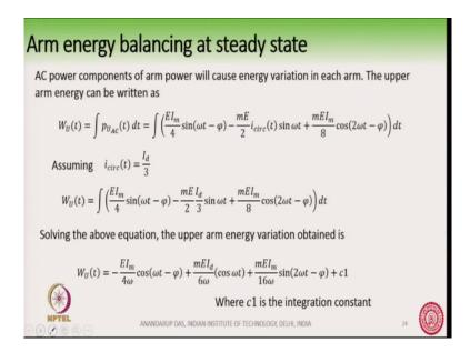
Now so, if we if we the upper arm energy so, what we will find out here is that this power causes a transfer of energy from the upper arm to the lower arm and from lower arm to the upper arm. Not only that the AC component of the power also causes the energy exchange from the one phase to other phase from a phase to b phase from b phase to c phase and c phase like that.
