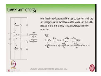
However, there is one point to be noted that and that is the when we started this derivation; we had said that this was the circuit diagram with which we started our derivation ok. Now if you note here that the direction of current and the polarity of the voltage here which we have assumed this is. So, for the upper arm, actually the current is flowing into the plus terminal.
