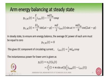
Yeah here, we have shown like the DC component of the average component of the arm power should be equal to 0. And that gave us this i circulating the expression of the DC component of the circulating current here. (Refer Slide Time: 02:28)
