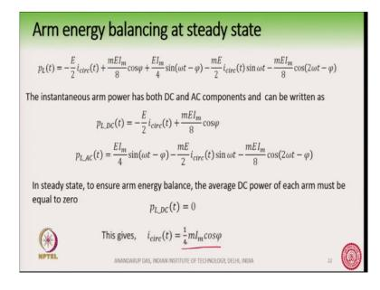
So, then this when you expand it fully, then again we see that in this lower arm power there is a DC component and there is an AC component just like before ok. So, this DC component again here, this DC component for the lower arm should again be equal to 0 to ensure arm energy balance for the lower arm.
