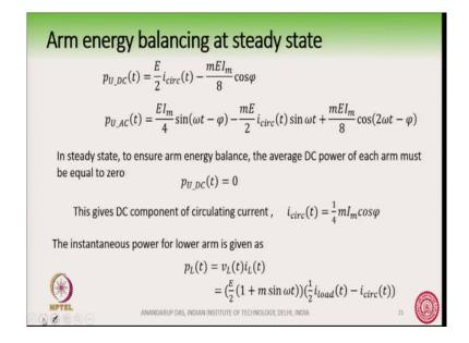
Now, let us collect the DC terms ok. So, what are the DC terms here? So, we collect this one here, this is the DC component and then we have the AC components here. So, we see that the DC component is this much and the AC component are these ones right these are the AC components.
