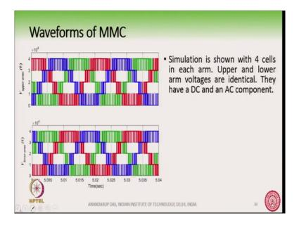
And accordingly the actual upper arm and lower arm voltages are something like this. So, since there are 4 number of cells you can clearly see the levels here. So, this is so that should be 5 levels because this is made up of half bridge. So, this is the first level 0 and there is a second level 1000 volt, 2000 volt, 3000 volt and 4000 volts right. So, each DC bus is 1000 volt there are a total DC bus voltage is 440 KV. So, each is 10 KV I was mistaken not 1000
