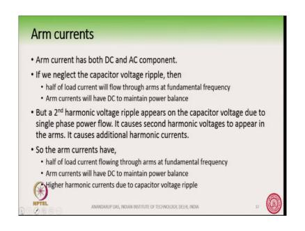
So, the Arm Currents have half the load current and a DC component these are essential, but then some higher harmonic predominantly second harmonic component which comes from the power oscillation due to a single phase voltage interacting with a single phase current. So, that comes also we will talk about it sometime later. (Refer Slide Time: 00:44)
