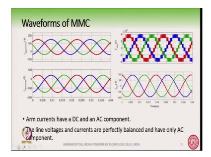
And the arm currents ok, so, this is the upper arm current and this is the lower arm current and this is the load current here ok. The load current is perfectly sin wave almost like a perfect sin wave with no DC component, but the arm current here both the upper arm and the lower arm you see these are shifted from the 0.
