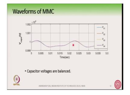
And the capacitor voltages; the capacitor voltages in these 4 cells these are pretty balanced ok, so, this is the 10 kilo volt. So, there are 4 capacitor voltages here probably you are not able to see the four distinct capacitor voltages here we see 1, 2, 3, 4 here there are 4 capacitor voltage, but they are pretty balanced actually there within the, there is a fluctuation here on the capacitor voltage, but they are pretty much balanced ok.
