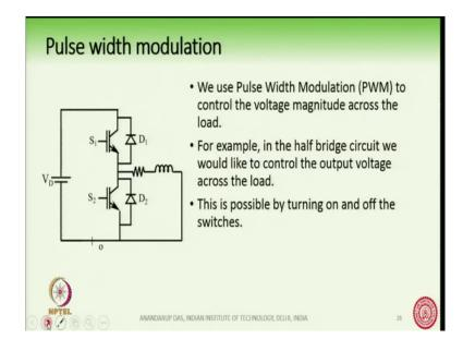
Now, before the next step in our analysis we will see what is called as a pulse width modulation. Why do we use pulse width modulation, because we want to control the voltage magnitude across the load. If you see here in for example, the full bridge the voltage magnitude across the load is always fluctuating between minus V D and plus V D and we cannot control the output voltage magnitude.
