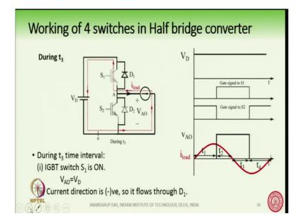
Next let us see the case during time interval t 3. So, we are looking now into this time interval t 3, during this time we see that the gate signal has been given to switch S 1 while the current is negative. So, since gate signal has been given to S 1 so, the either S 1 or D 1 will be conducting here.
