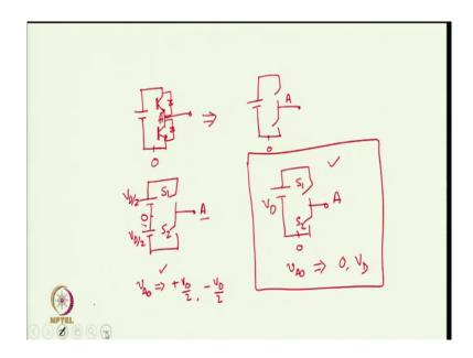
Now, if you analyze the 2 circuits for example. Suppose, we analyze these 2 circuits then we see that here the V AO voltage; the V AO voltage; the V AO voltage is always fluctuating between 0 and V D, where V D is this voltage here. the V AO voltage always oscillates or
