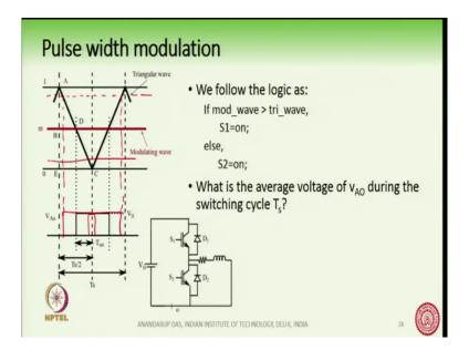
Now, we in order to control the output voltage of this half bridge we follow a logic. What is the logic? The logic is if the modulating wave is more than the triangular wave then I turn on S 1 otherwise I turn on S 2. So, let us apply this logic and see how the output voltage of the
