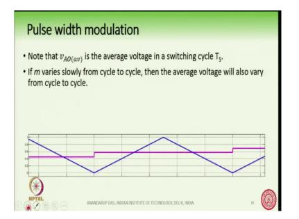
So, V AO average is the average voltage in a switching cycle T S which we have just now derived. Now, if we start to vary the value of m slowly from cycle to cycle ok. In this particular cycle which we see here the value of m is constant over the switching cycle, but suppose in the next switching cycle we just change the value of the modulating waveform slightly.
