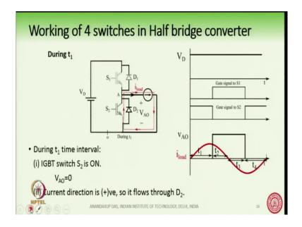
Here we have given the gate signal to S 1 and the gate signal to S 2 here. So, if S 1 gate signal has been given then the upper switch turns on the voltage between point A and O will be like this here, suppose the current waveform is alternating in nature. So, sometimes the current is positive and sometimes the current is negative.
