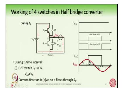
Now, let us take the second interval t 2 here, during the time interval t 2 we see that we have given gate pulse to S 1 while the current is still positive, if this is the case then we see that we have given the gate signal to S 1. So, which means either S 1 or D 1 will be on and since the current direction is positive.
