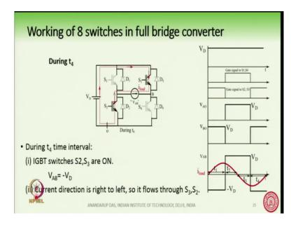
In a similar way you can also do the analysis for other durations. For example, if you take the t 4 duration you can make a similar analysis and can find out that the switches S 3 and S 2 are conducting just like how we have done with a half bridge. So, in this fashion it is possible for us to know all the 8 switches that 4 transistors and 4 diodes how they are conducting in this full bridge converter, ok.
