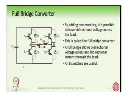
Now, so far we have analyzed the half bridge circuit; now, let us add one more leg to this converter which is called in fact, the full bridge converter. So, here you see that we; so, this is one half bridge and we have added one more half bridge to the circuit. Note that these 2 half bridges are completely independent of each other in fact, they do not know their existence they are just operating independently. So, the left hand half bridge does not know about the right hand half bridge.
