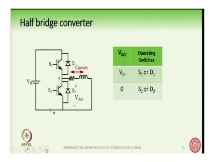
So, in this Half bridge converter we see that the switch S 1 or D 1 or the switch S 2 and D 2 may be conducting. So, how do they conduct, it is shown in this slide.
