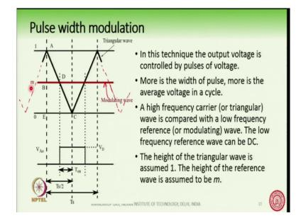
So, let us see how we can develop this pattern. So, in this pulse width modulation technique the output voltage is controlled by a series of pulses of voltage. So, if the pulse width is more, more is the average voltage across the load or more is the output voltage of the converter.
