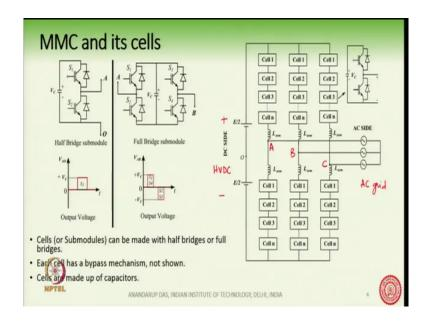
So, in HVDC application for example, at plus minus 400 kilo volt and say 800 mega Watt of HVDC application, we can connect hundreds of cells in cascade in an MMC converter. So, we can now see that this arrangement of series connection of cells is not limited to just a few cells connected in series. We can have hundreds of cells connected in series and so, the concept of modularity scalability is very much applicable for the MMC application.
