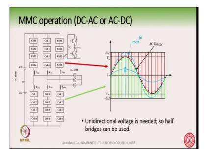
So, let us see the waveforms ok. Now, in this waveform whatever mathematical analysis we did has been now shown graphically. So, suppose this is the AC voltage which we are trying to produce this is the AC voltage you can see the peak of the AC voltage is V m here V m; the
