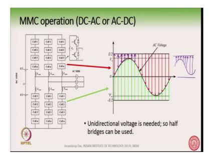
So, if I if I if this if this arrow waveforms are if the arrow wave arrow directions are made like this the opposite part like this, then if this AC voltage is available then it is possible that the DC voltage will be produced at the output of the converter. So, if we can flip the direction of the arrow, which means the controllable voltage source in the arms the controllable voltage source in the arms are now commanded to produce a voltage like this like this here.
