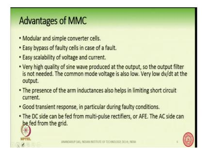
So, just summarizing the advantages of the converter. It has modular and simple converter cell like a half bridge bypass of faulty cells is possible easy scalability of voltage is possible and very high quality of sine wave is produced at the output. This we will see in the next slide how the sine wave is produced.
