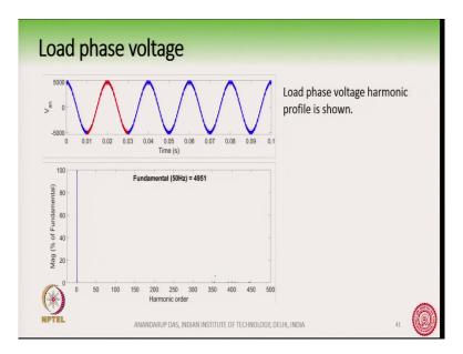
So, the load phase voltage exactly like before the harmonic side bands exists around 400 here and the triple n harmonics have disappeared, triple n harmonics have disappeared here and all harmonics at 400 times the fundamental. (Refer Slide Time: 18:08)
