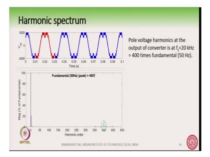
So, the harmonic spectrum if you see its again similar ok. So, the pole voltage harmonics again the output voltage is 4951 volt and the fundamental is kind of 100 percent, there is a
