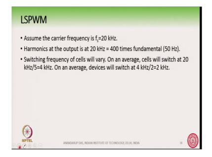
So, the level shift PWM; so, let us take an example just like the previous one assume that the carrier frequency is 20 kilo Hertz ok. Now, the harmonics at the output in level shift PWM will appear at 20 kilo Hertz that is 400 times the fundamental. Now, the carrier frequency here is itself 20 kilo Hertz. So, note the difference between phase shift PWM and level shift
