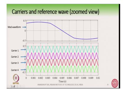
And, here we have shown a zoomed view of the carriers where you can see that these 4 carriers here is they are identical ok, unlike the phase shift PWM. In phase shift PWM these carriers were slightly phase shifted. But, in level shift PWM we see that all these 4 carriers are perfectly exactly same, but they are vertically shifted from each other and that is why it is called level shift PWM.
