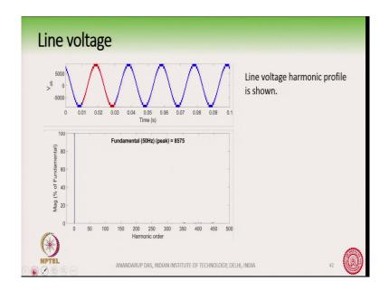
Line voltages also does not have the triple n harmonics anymore, the line voltages root 3 times the peak phase voltage magnitude.
