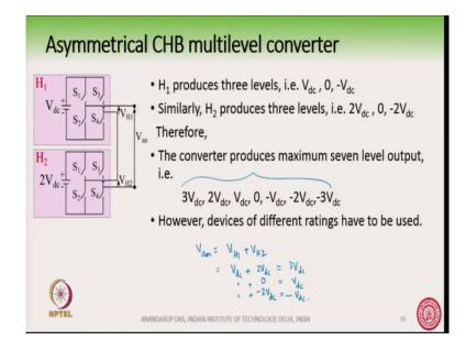
For example, we can make the voltage of H 1 V dc and that of H 2 of 2 V dc we can make it. So, then the how will V an voltage be; So, H 1 the first cell produces 3 levels which are V dc 0 and minus VDC.
