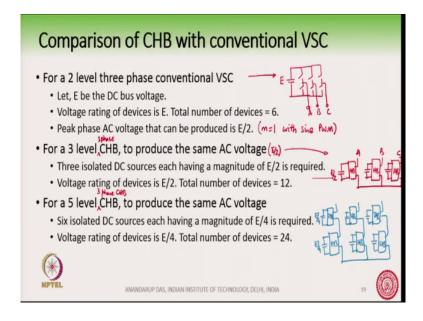
Suppose we make a comparison of the CHB with a conventional 2-level voltage; source convertor how do they compare with each other? So, this slide talks about that. So, suppose for a 2 level three phase conventional VSC which is this one ok, ABC here suppose. For this conventional VSC suppose if the DC bus voltage is E, that is this voltage is E then the voltage rating of all these devices are E and the total number of devices we require is 6 ok.
