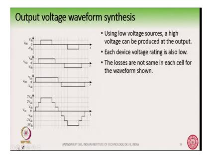
So, this is what I was talking about; using low voltage sources a high voltage source high voltage can be produced at the output where each device voltage rating is low. The one more
