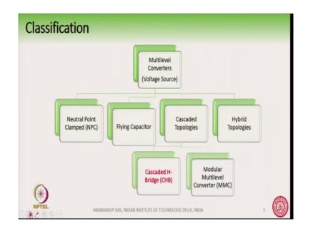
So, if we see the family of multilevel converters, basically this is multilevel converters are usually voltage source converters, we have this neutral point clamp converter in PC. We will study this in details sometime later. There is also this flying capacitor. Flying capacitor is, although it was commercially produced by one manufacturer, but it has not gained much success. So, we will briefly talk about this.
