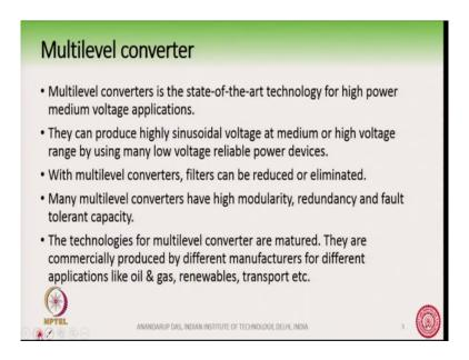
So, let us start with the multilevel converter. The multilevel converter is the state-of-the-art technology for high power medium voltage applications. It was introduced somewhere around the 80s, 1980s and slowly it became popular and the initially there were two types of multilevel converters, one was called the cascaded H bridge converter which we are going to discuss today and the other was the neutral point clamped converter.
