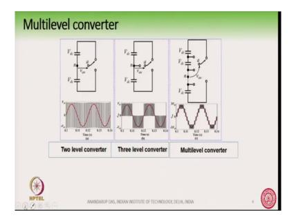
So, what is the basic idea of a multilevel converter? How does it produce sinusoidal wave form? This can be understood by this 3 diagrams here. Here on the left we have this two-level converter, then we have something called as a three-level converter and then we have a something like a multilevel converter.
