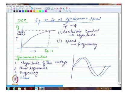
So first of all we talk very briefly about OCC or open circuit characteristics. Which we actually said in, talked in greater detail in a DC machine even in synchronous machine it is almost similar. So OCC is the voltage generated per phase or line to line voltage either way is fine versus I<sub>f</sub> at synchronous speed. So if I say that at synchronous speed if I am running my prime mover and I am trying to look at what is the generated voltage versus field current that gives me the OCC.
