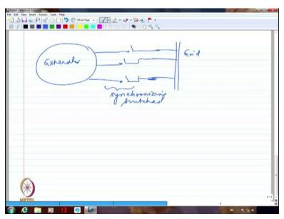
So let us probably slightly take a look at the synchronization process how it is done for smaller generators. From the generator I have 3 terminals, which are the armature terminal. Here is my grid, I am going to show this as the grid from which I am also getting 3 terminals. What I am looking at is to close these switches, this switch is closed, this is the second switch which I want to close, this is the third switch which I want to close. So these switches are synchronizing switches.
