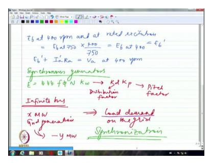
So E<sub>b</sub> at 400 rpm and at rated excitation =  $E_b$  at 750rpm \*  $\frac{400}{750} = E_b$  at 400rpm =  $E_b^l$ .
