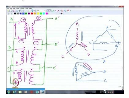
So, let us say I have one single phase unit something like this. So, this is one single phase unit I am showing, right and I am assuming that I am actually looking at the voltage rise in this particular direction, so I am going to mention this as dot, generally the dot indicates the polarity of one winding visa-viz the other winding. So, the other winding if I show again a dot here that means if I call this as positive with respect to this, this will also be positive with respect to this.
