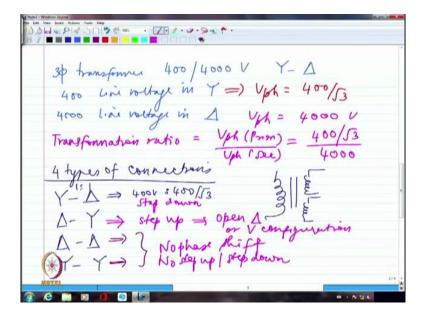
So, if we go back to our original configuration of delta-delta and star-star. These two will neither have step up, nor have stepped down inherently because they will translate exactly whatever voltage you are applying from the primary side into the secondary side. So, you are going to have essentially you know no phase shift at all in this particular case.
