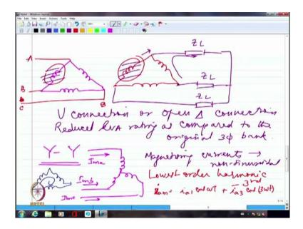
Similarly, if I look at  $i_{bm}$ . So let me write  $i_{am}$  here which is actually  $i_{am}=i_{a1}\cos\omega t+i_{a3}\cos3\omega t$ . Similarly,  $i_{bm}$  will be  $i_{b1}\cos(\omega t-120^0)$  because it is 3-phase. Similarly, this will have  $i_{b3}\cos3(\omega t-120^0)$ . And similarly,  $i_{cm}$  will be  ${}_{c1}\cos(\omega t+120^0)+i_{c3}\cos3(\omega t+120^0)$ .
