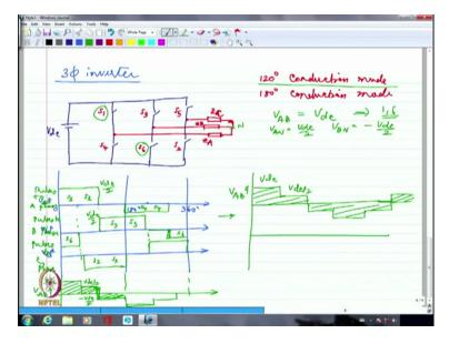
Professor:3 stages are because if I am not having any voltage at all in B. So, whatever is my A phase voltage that is returning through the third phase not through B. It is returning through C phase. So, B phase is not at all involved there is no current through B phase, so B phase is dead. So if I want to look at what is  $V_{AB}$  I have to essentially subtract  $V_{BN}$  from V<sub>A</sub>.  $V_{BN}$  is 0. So  $V_{AN}$  whatever is the value which is  $\frac{V_{dc}}{2}$  that is coming out.
