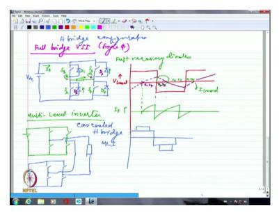
So, let us try to take a look at Full Bridge VSI. Again, we are talking about single phase. So, we are looking at a DC voltage source and then I am going to have 4 switches which is similar to that of whatever we studied in full bridge DC to DC converter, it is exactly similar and there will
