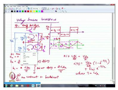
Now let us now go into VSI, voltage source inverters. So voltage source inverter let us start with first of all single phase half bridge. We had seen this already in the form of a half bridge DC DC
