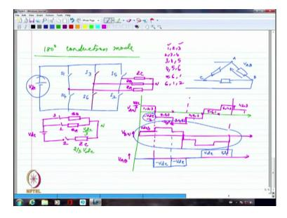
So in 180 degree conduction mode this is  $S_1$ , this is  $S_4$ ,  $S_3$ ,  $S_6$ ,  $S_5$  and  $S_2$  and we are going to have A phase, B phase and C phase star connected. Again, I am taking star connected loads. Delta and star normally would be a dual of each other, so please draw the waveform corresponding to Delta, a little later for 120 as well as 180. You would see that the phase voltages and line voltages reverse their rules. Actually, in terms of the shape what you get.
