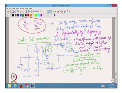
You can very well see that the expression is very much similar to the buck converter except turns ratio of the transformer. So we will be able to adjust in many of the isolated DC-DC converters, the output voltage can be adjusted right by appropriate design of  $N_2/N_1$  this is one way. The
