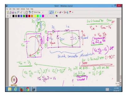
So let us now try to draw the circuit of the forward converter. So in the forward converter again I am going to have a primary which is connected to the source through a switch and I am going to have actually a secondary. The secondary is going to have one diode and I am going to have one more freewheeling diode and then I am going to have inductance which is going to smooth out the current. Then I am going to have a capacitor and I will have a load.
