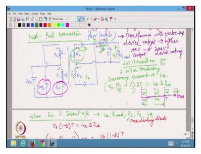
What I want to say is that, if you look at this entire operation,  $S_{w1}$  is going to be operated for  $D\frac{T}{2}$ . And  $S_{w2}$  will be operated for  $D\frac{T}{2}$ . So if I draw the wave forms I should show it as though
