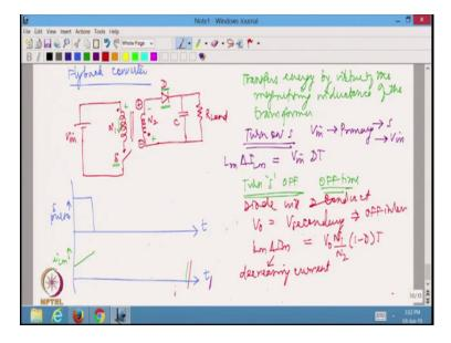
So we are looking at flyback converter, we have already drawn the circuit diagram. The output side has a diode, a capacitance and a resistance load. And the input side is having a switch and along with a transformer let us say this is the input voltage  $V_{in}$ . And let us say this is going to have  $N_1$  as number of turns and this is going to have  $N_2$  as the number of turns. This flyback convertor basically transfers energy by virtue of the magnetizing inductance of the transformer.
