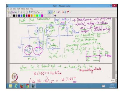
One more thing that we will have to realizes is that what I am applying here is  $V_{in}$ . So when  $S_{w1}$  is conducting, I am going to have this carrying  $V_{in}$  but the same voltage is going to be induced on the other side also because this is also having  $N_1$  turns.
