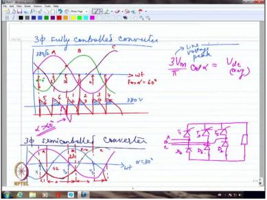
So we had stopped at the point of three-phase fully controlled converter. This is where we had stopped and I think I had drawn the waveform corresponding to  $\alpha=30,\alpha=60, \alpha=75$ , and then maybe 90, I said positive and negative sides will be exactly equal to each other due to which you will have 0 voltage. So if you may recall, let me again draw only corresponding to  $\alpha=60$ , then we will go over to semi-controlled converter.
