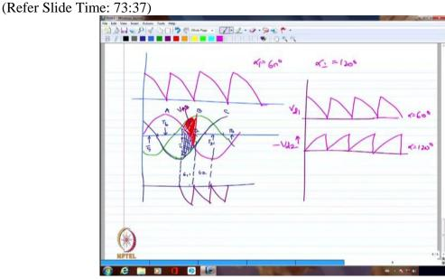
So if I try to do that, for example, let us say I am firing one at  $\alpha$ =60, we all now have at least I hope you guys have gotten familiar with this  $\alpha$ =60 degree waveform. This is  $\alpha$ =60 degree waveform, normally. If  $\alpha$ =120, what kind of waveform I have to get, I have to check. Let me
