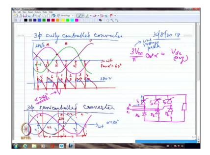
So please look at this circuit. So, if I have A, so if 1 is conducting, device number 1 is conducting, A phase current is positive. If device number 4 is conducting, A phase current is going to be negative. So, I have to look for wherever 1 is conducting, I will have correspondingly that particular current to be, A phase current to be positive. So let me take a look at this.
