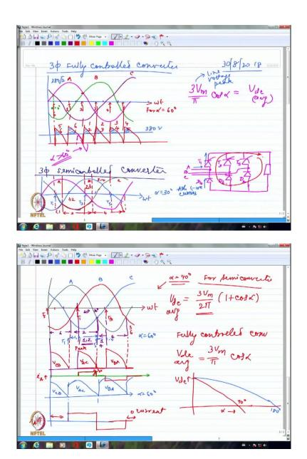
So if I am having for example, these 2 are freewheeling, I am going to have simply the current going like this. There is nothing that is going through the supply. It is just going round and round in this. That is it. So the supply will be deprived of any current or it will not carry any current during the freewheeling. So if I try to look at the current here in this particular case, I would see that for example, during  $V_{AC}$ , I will have a positive current.
