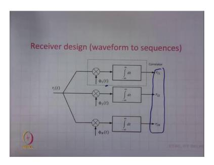
Similarly, we have looked into the receiver design. If we are receiving a waveform, we pass this waveform through what is known as correlator and at the output of the correlator, we have the projection of this waveform along this orthonormal basis functions. So, then we can obtain a sequence corresponding to the received waveform.
