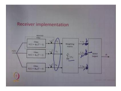
Then we have looked at the full blown receiver implementation where the receiver first produces the sequence corresponding to the received waveform and then, it does the inner product of this received sequence with the sequence of the signal set that it has. We have said if these signals are not of equal energy and they do not occur with equal probability, then normally you also have to add some bias.
