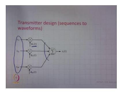
So, transmitter converts sequences to waveforms. If we have a sequence, we multiply each element of the sequence with orthonormal basis function and sum up all the products of this multiplier. So, from this we get a signal.
