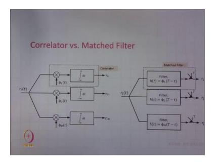
We have also said that instead of this correlator, which is made up of a multiplier and integrator, we can have a matched filter which is a filter whose impulse response is matched to orthonormal basis functions. So, we need to use a bank of matched filters or a
