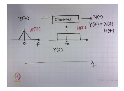
So, if I have a signal X t and let us say this signal has got a spectrum like this. So, centered at 0 and let us say that this I am trying to pass over a channel and channel has the spectrum centered at around f c what happens what is the output. So, you must have seen from signals and systems that the output spectrum is nothing, but it is the multiplication of input spectrum and the channel frequency response.
