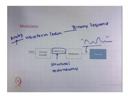
So, you know that we already have looked into the issues of waveform coding. So, waveform coder takes in analog waveform and this analog waveform is converted into binary sequence, then this binary sequence goes to channel encoder, channel encoder introduces some structural redundancy, introduces some structural redundancy in this binary sequence and modifies this binary sequence and this structural redundancy is introduced so, that the binary sequence is made more robust to channel errors
