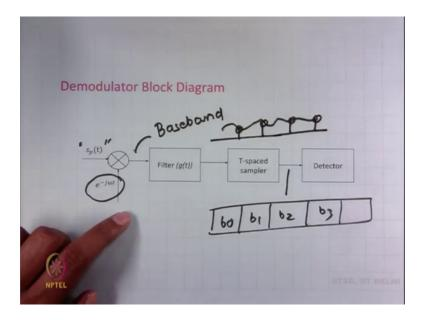
Let us look at the demodulator. So, now we have this passband waveform Sp t. Here I am showing that I have the same passband waveform which was available at the output of the modulator, but in reality channel will corrupt this. At this point I am assuming that I have the same passband waveform available at the input of a demodulator that was available at the output of a modulator.
