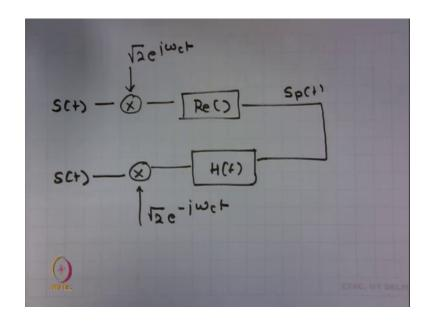
So, if we have a complex baseband signal let me multiply this with root 2 times e to the power j omega ct. Take the real part I get Sp t, Sp t I pass it through Hilbert filter which is like a unit to step in frequency. I multiply this with root two times e to the power minus j omega c t. I get S t.
