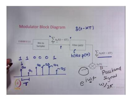
So, overall purpose is to take in the binary sequence and produce some analog waveforms. So, the first step is that you have this binary sequence or a sequence of bits and these sequence of bits are converted into sequence of samples. For example, if we have these bits what you can do is, you can have an impulse train. Do not worry about the correctness of this mapping. The only thing that I am emphasizing at this moment is what typically happens in this bits two samples converter.
