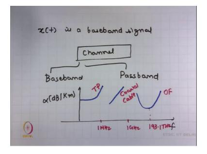
So, the information signal xt is a baseband signal and the channel can be a baseband channel or it can be a passband channel. We have also seen these issues in lecture 6. For example, in the case of wired we have already plotted the attenuation was this frequency curve. Let me plot it again.
