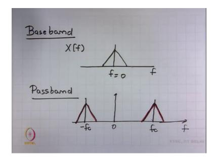
Let us first start by revising the definitions of baseband and passband signal. So, remember we have already talked about this. I am just revising it. So, baseband signal is a signal whose spectrum is centered at around dc. That is the baseband signal and we
