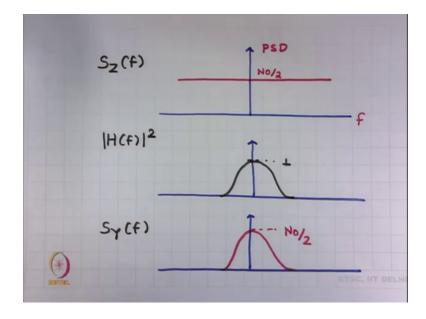
For example, if you have this as the power spectral density of the input random process, particularly in this case we are talking about white Gaussian noise. So, white Gaussian noise has this power spectral density. If it passes through a filter whose mod square of frequency response is such a response, then the output power spectral density is shaped by this function.
