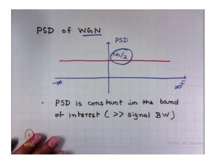
So, what we are saying is the power spectral density of a white Gaussian noise which is abbreviated as WGN. So, it is a very common abbreviation. You should get familiar with this abbreviation WGN. W refers to White; G refers to Gaussian and N refers to Noise. So, the power spectral density of a white Gaussian noise is constant ok.
