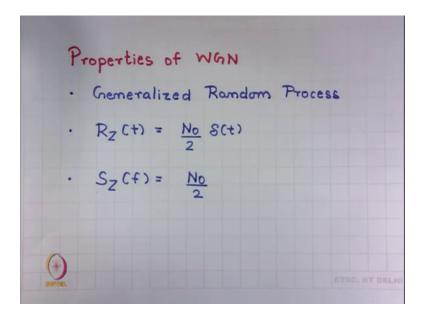
So, what are the properties of white Gaussian noise that is the next question? And the properties of the white Gaussian noise is, it is a generalized random process. It has an auto correlation function which is N naught by 2 times delta t. It has a power spectral density which is constant, and the value of this constant is N naught by 2.
