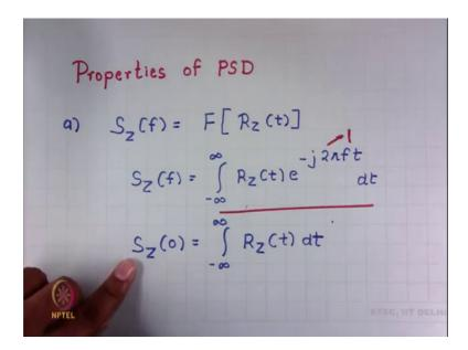
So, if we look at these expressions, the power spectral density is the Fourier transform of a autocorrelation function. So, you know that this gives me the Fourier transform of a quantity. And furthermore if I put f equals to 0, and use something like moments theorem, then this goes to 1. So, we end up with this. That means, we are saying if you take the area under the autocorrelation function, you get the power spectral density at frequency 0. So, this is an important idea which you can use.
