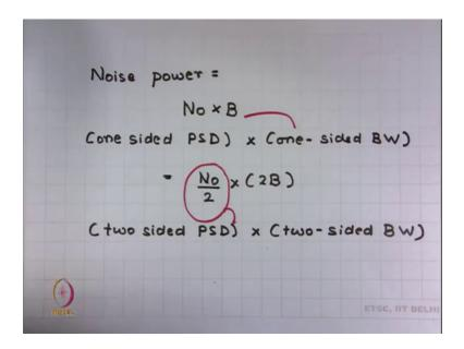
So, what we are saying is noise power available at the output of a filter is N naught times B, we have already seen that this B is refer to as one-sided bandwidth. So, while thinking about the one sided bandwidth we have only to look at the positive side of the spectrum and this n naught is one-sided power spectral density.
