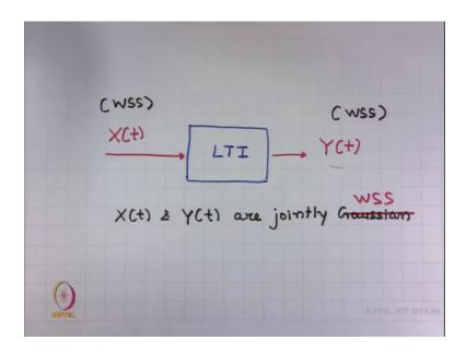
And we looked into what happens when a wide sense stationary process let us say x t passes through a linear time invariant systems, we said and we have seen that the output process also remains wide sense stationary. And we have seen that these two processes are also jointly wide sense stationary processes ok. So, this is what we discussed in the last lecture. Let us see what we have to cover today.
