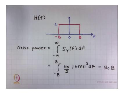
Finally, the last point where we will like to talk about this noise power and try to understand the idea of N naught by 2 is let us now pass this noise through this filter, this is a rectangular shaped filter whose magnitude is 1, and it has a bandwidth of B. So, noise power can be obtained by integrating the output power spectral densities.
