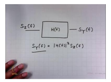
Final point, what happens if you pass this white Gaussian noise through a filter? We already have seen that the output power spectral density is nothing but the input power spectral density multiplied by mod square of the frequency response of the filter. And this property can be used to generate Gaussian random processes with different power spectral densities. You can really manipulate the power spectral density of the Gaussian random processes.
