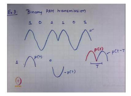
So, when we are talking about a binary PAM signal, let us assume that I have some digital signal and this digital signal as you can see is composed of two bits 1 and 0. Let me assume that to transmit 1 I use a pulse shape like this and to transmit 0 I use a pulse
