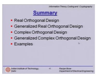
So, let us now try to conclude what we have studied in today's lecture. We started out with the notion of real orthogonal designs which provide single symbol decoding and full diversity and we realize that only N is equal to 2, 4 and 8 is possible for real orthogonal design that motivated us to look at generalized real orthogonal designs, where we are working with a matrices which are not square and so, you can have more number of time slots.
