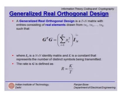
So, what is the definition? A generalized real orthogonal design is a T cross N matrix. So, if you have to design a generalized real orthogonal design we have to just come up with a matrix which is T cross N, but all the elements of this matrix all the entries are real drawn from plus minus x 1 plus minus x 2 up to plus minus x K such that G transpose G is again equal to I is equal to 1 through K x i squared I N, where IN is a N cross N identity matrix, ok.
