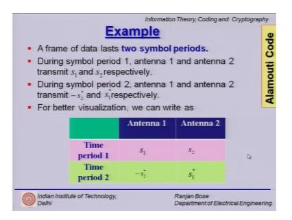
So, in this example we have talked about the space antenna 1 and antenna 2 and time; time period 1 and time period 2, so, we have this matrix of symbols that we want to transmit and this is kind of the code the space time block code that is being used.
