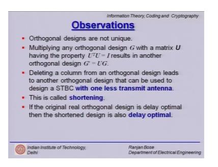
So, some observations orthogonal designs are not unique, number -2 multiplying any orthogonal design G with a with a matrix U, right having the property U transpose U T U equal to 1. So, results in another orthogonal design ok. So, deleting a column from an orthogonal design leads to another orthogonal design that can be used to design a space time block code with a one less antenna.
