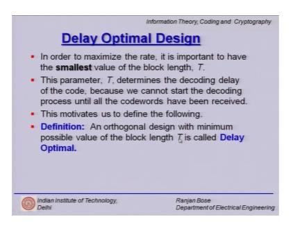
Now, let us talk about delay optimal design. Clearly as we increase the size of T, I will use more and more time slots if I use more and more time slots then my delay would increase at the receiver side to get the decoded output. So, let us talk about this delay optimal where we minimize this T. So, in order to maximize the rate it is important to have the smallest value of the block length T, this is obvious.
