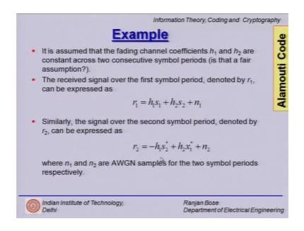
And, we can multiply it out to get the first received signal in time slot 1 as a r 1, this is simply s 1 with channel gain h 1 plus s 2 with channel gain h 2 plus n 1. Similarly, in the second time slot we have minus h 1 s 2 star plus h 2 x 1 star plus n 2 here it should be s 1. So, we have this received signal r 2 in the second time slot. Now, the observation right here is that r 1 depends both on s 1 and s 2 and r 2 also depends on s 2 and s 1, simultaneously.
