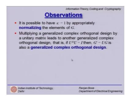
So, it is possible to have kappa is equal to 1 by appropriately normalizing the elements of G is still remains an orthogonal matrix and we can multiply as before with the unitary matrix then G prime equal to U times G is also generalized complex orthogonal design. So, multiplication by unitary matrix as in the earlier case does not change it is still remains a generalized complex orthogonal design.
