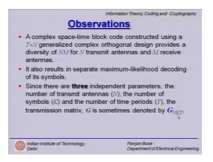
So, some simple observations a complex space time block code constructed using a T cross N generalized complex orthogonal design provides a diversity of N cross M. So, N is the number of transmit antennas M is the number of receive antennas. So, this is the diversity that is provided and it also results in a separate maximum likelihood decoding symbol by symbol decoding is possible.
