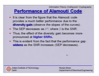
Then, we can go and find out how the diversity gain is obtained from the Alamouti code. So, diversity gain is obtained simply by looking at the slopes of the BER curves. So, on the x axis we can have the SNR, y axis we have the symbol error rate, if you will and then if you look at with and without Alamouti code you see a distinct change in the slope which indicates the a diversity gain.
