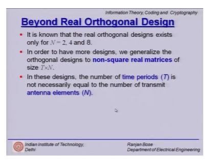
So, it is known that real orthogonal designs exists only for N N is equal to 2, 4 and 8. So, how do we go beyond that? We have to generalize the orthogonal designs to non square real matrices of size T cross N earlier it was N cross N, but suddenly I want to have T which means I want to increase the number of time slots. So, it might take a hit on the rate. So, the number of time periods is denoted by T and the number of antenna elements is N and T is not necessarily equal to N.
