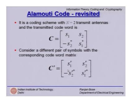
So, we quickly revisit the Alamouti scheme with N is equal to two transmit antennas and this is the code further Alamouti scheme and if we have another pair of symbols and this matrix is denoted by C prime as follows.
