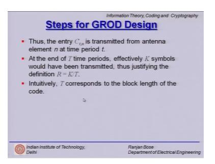
So, thus the entry C t comma n of the code is transmitted from the antenna element n at the time period t, that is the notation. At the end of T time periods effectively K symbols would have been transmitted, thus justifying the rate R is equal to K by T.
