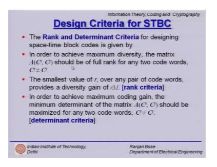
In the last class, we therefore, came up with this rank and determinant criteria for designing space time block codes and what we came up with is the rank and the determinant criteria. So, we defined this matrix A and we said that it should be full rank for any two code words C i not equal to C j and the smallest value of the r rank over any pair of code words provides a diversity gain of r into M, where M is the number of received antennas.
