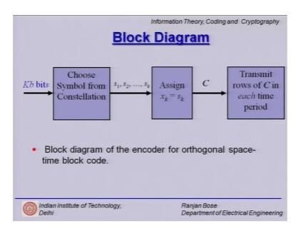
Let us show it using a block diagram for orthogonal space time block codes. What we have done is taken K bit bits coming at a time divided this Kb bits into b bits then b bits then b bits and so and so forth for each of the b bits I pick up one symbol from the constellation diagram.
