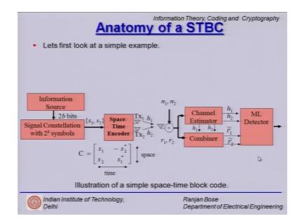
Let us revisit the anatomy of a space time block code STBC for short and what we realized was that an information source pumping in bits of information what we do is we take 2b bits at a time and of this first b bit is used to select one signal from the signal
