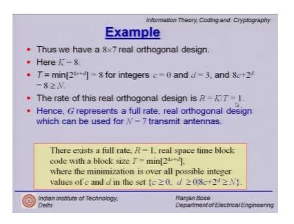
But, we also see that 8 cross 7 is a real orthogonal design with K is equal to 8 and you can do T as minimum of 2 raise power 4 c plus d equal to 8, because the integers which we found was c is equal to 0 and d is equal to 3. So, we have satisfied those conditions and we were able to get this 8 plus 7 matrix. So, not only it tells you that this T cross N matrix exists, but you already have an example of what that matrix should look like.
