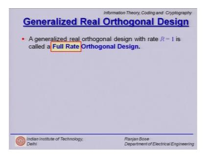
But of course, in real life we would like the rate to be as close to 1, if not 1. So, a generalized real orthogonal design with rate R is equal to 1 it is called a full rate orthogonal design, ok; so, if we are still in the domain of generalized real orthogonal design, but we are not talking about full rate design.
