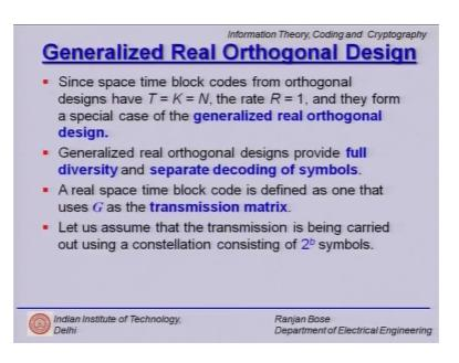
Since the space time block codes from orthogonal designs have to have T is equal to K is equal to N and the rate R is equal to one and they form a special case of the generalized real orthogonal design. So, the already the case of N is equal to 2, 4 and 8 the orthogonal
