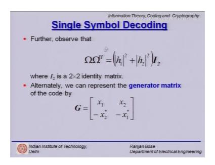
So, you observe that this sigma sigma Hermitian is nothing, but h 1 squared plus h 2 squared I 2 and the generator matrix for the code is simply given by G. So, throughout this lecture this is how we will denote the generator matrix of the code for different cases. This is a 2 cross 2 complex design, but we will look at real designs and complex designs in our subsequent slides.
