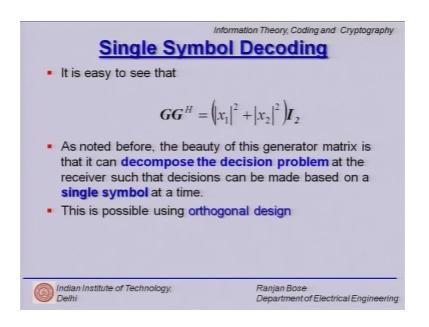
So, what is interesting about this generator matrix is if you take GG Hermitian you come up with a scaled identity matrix and this interesting fact allows us to decouple the decoding problem and we do symbol by symbol decoding we have one single symbol at a time which is required to take the decision. And the reason is because we have an orthogonal design. So, GG Hermitian is simply this identity matrix multiplied by this term.
