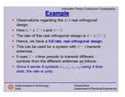
So, what are the observations regarding this design? T is equal to 4, N is equal to 3, as we observed K is equal to 4, but the rate is 1, ok. We did not compromise on the rate. So, it is a full rate generalized real orthogonal design. So, we have only used 3 transmit antennas because N is equal to 3, but we have judiciously used the 3 antenna elements in different time slots to send out the message which are single symbol decodable.
