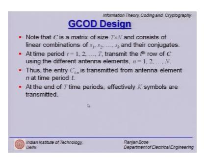
So, this C matrix is of the size T cross N and it has a linear combination of s 1, s 2, up to s k and their conjugates because it is a complex design. So, at time period t is equal to 1 through T you transmit the t-th row as before and then, clearly the C t comma n is transmitted from antenna element n at time period t as before it is pretty much the same and we have transmitted effectively K symbols at the end of T time period thereby justifying that rate.
