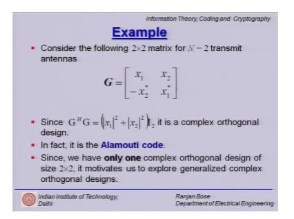
This is an example of a 2 cross 2 matrix which we have already seen as being an orthogonal design it is the Alamouti code, but this is the only one complex orthogonal design which exists size 2 cross 2.
