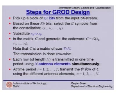
So, pick up a block of Kb bits coming from the input stream. So, we have no worries getting enough bits to process today we are generating humongous amounts of bits, but what we do is we take up a block of K into b bits. Remember, the constellation has signals coming from 2 raise power b points in the constellation.
