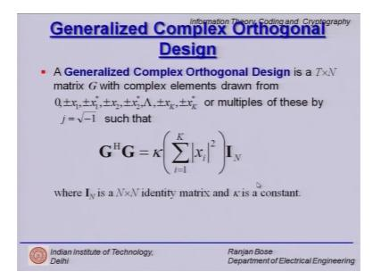
So, we define it quickly. Generalized complex orthogonal design similar to the generalized version of the real orthogonal design is a T cross N matrix G with complex elements drawn from 0, x 1, x 2, x 3 and so and so forth up to x K such that G Hermitian
