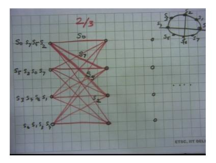
There are 4 states in the trellis, because if you see you have 2 memory units leading to 4 states and it is a fully connected trellis which means that each node is connected to every other node and so and so forth. Now for any bit that comes in and this is a rate 2 by 3; so 2 bits come out so they have possible 4 possible transitions 0 0 comes in take this branch, 0 1 take this branch, 1 0 take this branch, 1 1 take the last branch.
