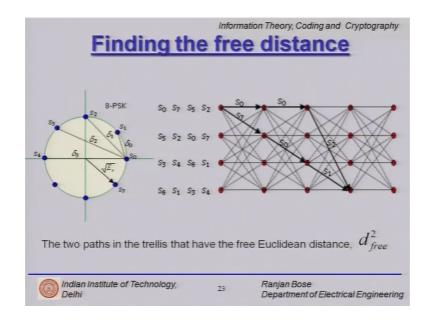
So let us look at this diagram and this is the same trellis coded modulation scheme described earlier here after a lot of inspection we have been able to identify 1 pair of path which leads to the minimum distance called the free distance.
