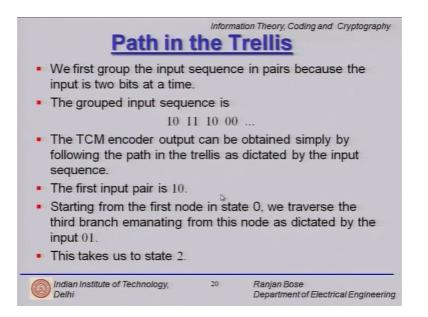
So, if you look at the path in the trellis this slide tells me how to go from the input sequence to the path on the trellis and the encoder takes 2 bits at a time and follows the consequent paths in the trellis.
