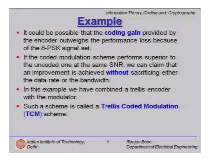
So please note we did not sacrifice data rate in either case we got those 2 bits per second through the channel. So in this example we have combined a Trellis encoder with a modulator and hence we have looked at combined coding and modulation; this scheme is called a Trellis Coded Modulation or TCM for short.
