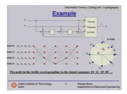
So, here is in a nutshell all of it if you see this is the hardware followed by the mapping, so I can describe my TCM scheme as a diagram with a circuit implementation and a mapping or equivalently I can define my trellis using the states and a trellis diagram they are the same you give me 1 and I will give you the other.
