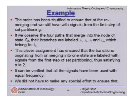
So we have done all of this and the order has been shuffled to ensure that the re the at the reemerging and we still have the signals with the first step of the set partitioning that is the care we have taken to do so and we have also ensured that the all the symbols have been used with equal frequency.
