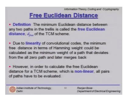
We have looked at free distance earlier in terms of convolution codes we define the free Euclidean distance; so the minimum Euclidian distance between any 2 paths in the trellis is called the free Euclidean distance d free of the TCM scheme. Please note here since there is a convolution encoder present they will be a trellis diagram, but the labels of the branches instead of being bits should be symbols because, all the bits have been mapped to symbols.
