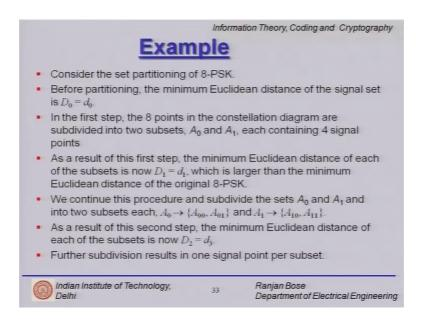
So, now the aim is how to use this partitioned set and map it to the trellis that we have here; so what we do is we basically come up with a rule as to how to apply these points from the different levels of constellation diagram because level decides what is the minimum distance in terms of the diverging and merging paths.
