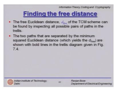
So, now we go to the job of finding the free distance; we know that free distance is the single most important parameter which describes how good this trellis code is. So the free Euclidean distance of the TCM scheme can be found by inspecting all possible pairs of path in the trellis not just from the all 0 path this is because we are dealing with a non-linear code.
