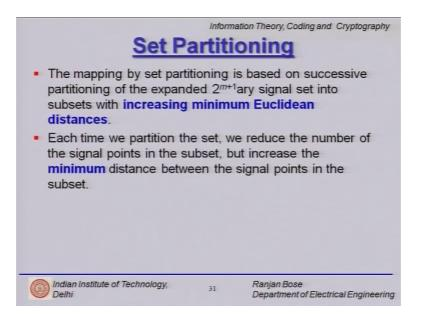
So, the aim of set partitioning is to progressively increase the Euclidean distance and then use that partitioned set to map onto the trellis; each time we partition the set we reduce the number of signals points, but increase the distance between the signal points in the subset.
