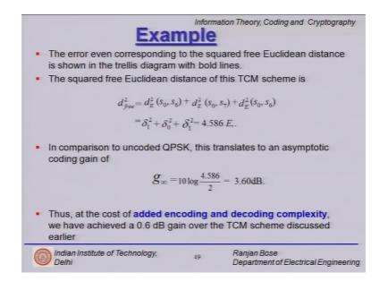
Lets quickly calculate the d free, so d free we had already highlighted the 2 paths which result in d free and the d free calculation gives the g infinity 2 3 point 6 db therefore, this has a even better point 6 db gain over the TCM scheme discussed earlier by Ungerboek.
