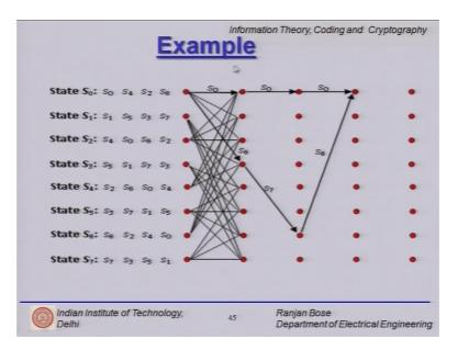
So, this is a trellis with 8 states and as you can see that there are 4 branches emanating from every node ok. So that 2 bits coming in for this convolutional encoder and there are clearly s 0 to s 7 so there are 8 points in the constellation diagram so 3 bits are being mapped to the symbols so it is a rate 2 by 3 encoded that has resulted in this trellis.
