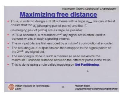
So, it will not be a bad choice so we look at the diverging d E diverging path and reemerging path and we have a redundancy of 2 raise power m plus 1 m-ary signal set is used to transmit m bits; why because we had this 8-PSK and then we went to from QPSK we went to 8-PSK.
