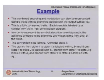
So, if you see that this combined encoding and modulation can be represented using a trellis diagram, but this time we label the branches with the output symbols and this is a fully connected trellis where each branch is labeled by the symbols from 8-PSK and encoding is a simple process as we had learnt earlier; 1 comes in you take the upper branch, 0 comes in take the lower branch and you read out what is written on top of the branch.
