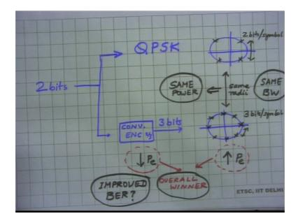
But we say no wait a minute this 2 bits can be passed through a convolution encoder which is rate 2 by 3, so 2 bits go in and 3 bits come out.
