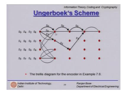
And for that we are going to do an Ungerboeck scheme and here you can see that there are parallel paths in this case because you know if this input a 1 does not change then the state transition does not change and for a 2 between 1 and 0 there are 2 possible outputs so there will be 2 paths from any 1 state to the next state, but the question is how to assign the symbols from the 8-PSK.
