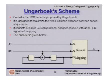
Now, we go on to Ungerboek scheme which tells us how to assign the symbols on to the trellis having done the set partitioning so the aim is to maximize the free Euclidean distance between coded sequences so just consider an example of a rate 2 by 3
