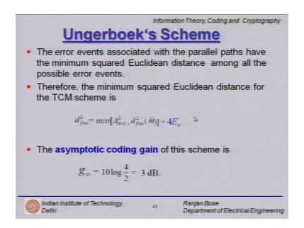
So once you do a mapping as described earlier then we can calculate directly the d free as the minimum of delta square m tilde plus 1 and d free squared m tilde which is E 4 comes from the maximally separated points on the symbol set and this tells you that the d free is larger than the uncoded one giving us an asymptotic gain of 3 db. So we have been able to recover and we have been able to give you a 3 db gain using a TCM scheme this called the Ungerboek TCM scheme.
