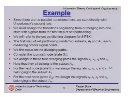
So, there are no parallel transitions we start directly with the Ungerboek second rule of assigning; so in this trellis we have assigned s 0 s 4 s 2 and s 2 from for these 2 for these 4 branches which are diverging out.
