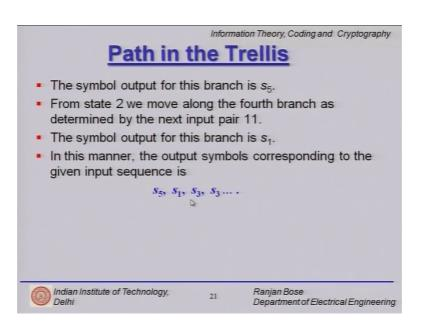
And reads out the corresponding symbol written on top of that branch so this slide basically tells you that first branch has s 5 written on it so read out s 5 second branch has written s 1 on it so read out s 1 s 3 and s 3 and so on and so forth.
