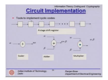
So, here are some of the tools that we use the circuit hardware tools, so you have the n stage shift register, we have a scalar multiplier, we have a simple adder and a
