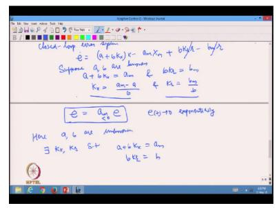
So if these 2 conditions are true, then e dot becomes equal to simply  $am^*e$ , right. Because these 2 terms cancel off and this is what we get, okay. So e dot, right. So this is a stable linear system since am<0. So e will exponentially converge to 0, right. And here what is the condition? The condition is that we choose Kx=am-a/b and we choose Kr to be = bm/b. This is similar to the case that we had discussed when the parameters are known, okay for the mass spring damper case.
