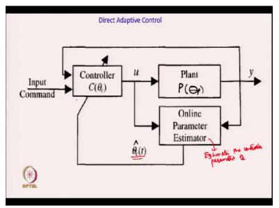
Let us move on to the direct adaptive control approach. So, so in this approach, the idea is very similar that an online parameter estimator has to be used. But here the online parameter estimator directly estimates the controller parameter. So this estimator estimates the controller parameters theta c. So let us call this, that estimate as theta c hat and again as you can see it is a function of time.
