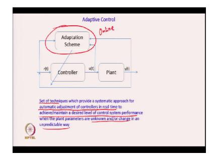
So what I mean to say is that here what we do is we construct a controller for this plant and then we have an adaptation scheme here. So this adaptation scheme has an inbuilt logic, an inbuilt strategy to, to adjust the parameters of the controller, okay. So the adaptation scheme's input are the input to the plant, the output of the plant, the desired trajectory or the desired reference signal and it has some way of adjusting the parameters of the controllers online.
