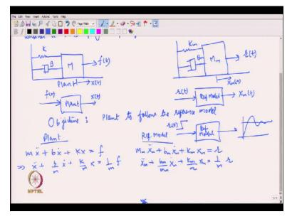
So by the way the mass spring damper system can be used to model many physical systems, example the suspension of the car. The main examples are you can find that where, whereever you have an inertia, a storage element, a dissipation element, these mass spring damper systems can be used to model such systems, okay. So it is, it is a practical example that we have considered and the task is for, for this plant to, to have a desired closed loop response.
