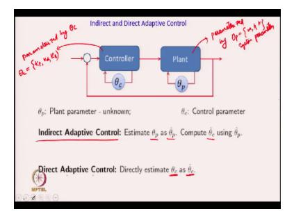
One is the indirect adaptive control and the other is the direct adaptive control. So I want to talk about them in brief. So let us again consider this plant which is parameterized by the parameters theta p. So for the mass being damper case for example, here you would have m, b and k as your parameters of the plant and let us denote all of them as theta p which we call as the system parameters.
