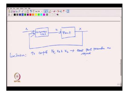
And so we, how we could reprint this as a, as a control system is we are trying to control this plant and it is, and the controller that we have used is simply Kp\*X+Kd\*X dot+Kr\*r, right, that is the controller that we have used and the output of the plant is X, the input is u. So X is goes to the feedback and we also have the reference signal r. So this reference signal is the same signal that is the input to the reference model, okay.
