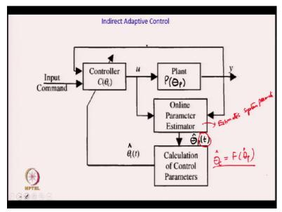
I have a block diagram of the 2 approaches. So let us just, in brief, go through them. So as I mentioned the plant here is parameterized by, by theta p, the controller is parameterized by theta c and in the indirect adaptive control approach, we use the input to the plant and the output of the plant as input to an online parameter estimator, okay which, which estimates, for the indirect case, it estimates the system parameters and so it online estimates the system parameters.
