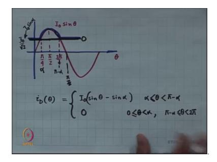
Let us say this is some I naught sin theta, ok. This is the sine wave. Now, we are going to draw a line and above that line, it is going to conduct, below that line it is all going to be 0. In such a case, our line is going to be at 45 degrees. This is the line, fine. What is the value at that line? I naught sine pi by 4 which is I naught by root 2, alright. Above, that it is going to conduct; below that it is we are not going to bother.
