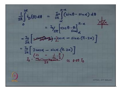
So, its 1 by 2 pi integral 0 to 2 pi i D of theta d theta, but in our case i D of theta is mostly 0, it is mostly 0, its non zero only during this angle right. So, all that we have to do is 1 by 2 pi integrated from alpha to pi minus alpha.
