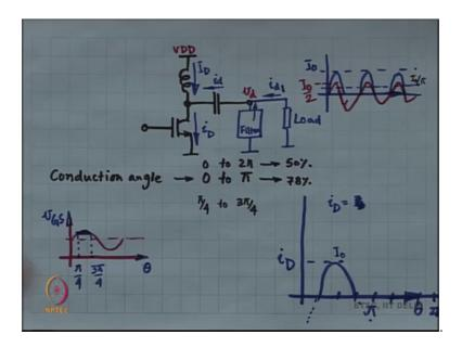
So, single transistor, huge inductor, huge capacitor, this one circuit for the power amplifier, all that we are tweaking is the gate bias voltage. So, in the last class we had kept the gate bias voltage, such that the MOSFET conducts only for half of the duration.
