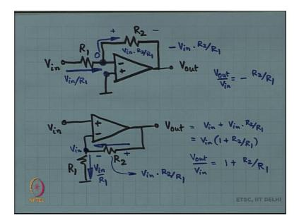
So, one was this and the other was variation of that and, the analysis of these circuits is very straight forward, all you have to remember is that, if you are drawn the circuit right, then the voltage at minus terminal is going to be equal more or less equal almost equal to the voltage at the plus terminal ok, which means that the voltage at the minus terminal in this particular circuit is 0.
