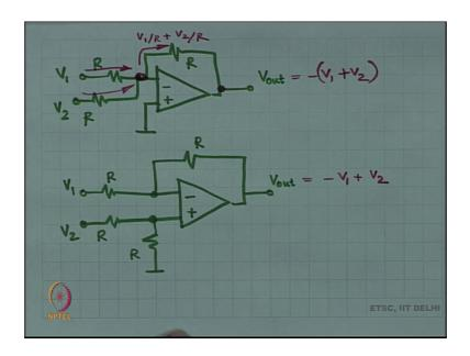
So, for example so, what is going to happen here, if there is negative feedback, then the minus terminal will be equal to the plus terminal that is the idea number 1. If there is negative feedback minus and plus are going to be equal, if they are equal in this case there is negative feedback.
