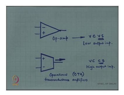
You think the op-amp is going to work like a voltage source right voltage controlled source it is going to amplify the difference between plus and minus by very large number and give you corresponding voltage at the output. So this is ordinarily what we think of as the op-amp, but does it matter if it is a voltage source or a current source.
