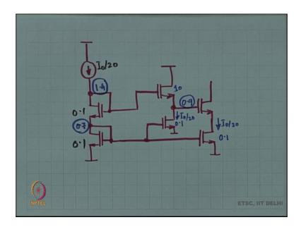
By the way these 0.5, 0.2 these are just numbers that I have picked up from my head in reality it would not be 0.5 and 0.2, in reality you will need v gs minus v t may be of 250 millivolts, 150 millivolts something v t could be 0.5 v t could be 0.4 it could be 0.3 it could be 1 volt whatever it is right.
