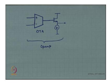
So, you take this OTA which is what we have made and then if you wanted to make an op-amp then we need to have a buffer stage which has a low output impedance. What is a buffer stage? Something like a common drain amplifier, where is this common drain amplifier coming from.
