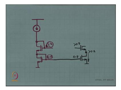
So, I am just drawing this branch all right just this portion. If I do the regular Wilson, this is the regular Wilson I was getting 0.5 plus 0.2 so 0.7 over here and 0.7 plus 0.5 plus 0.2 so 1.4 over here and that was too much ok. We need to change the structure any voltage over here within some bounds is all right what are those bounds?
