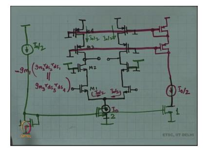
And then, yesterday, in the last class we were working on this differential cascode amplifier we said that the small signal circuit is just like the small signal differential mode half circuit is just like the regular cascode amplifier. In fact, it has to be the same, right that is the entire point, ok.
