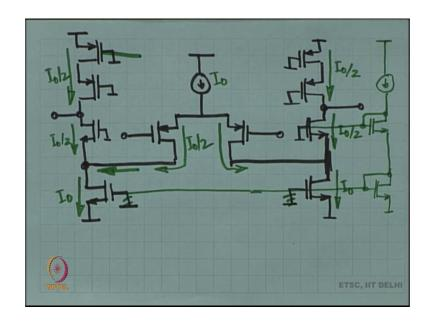
So, these are my two inputs I am sorry ok. So, the first thing you should notice is that my stacks size has reduced, I have now got a stack only of four transistors, ok. This is not the complete thing, this is still the small signal incremental picture I have converted the differential half circuit into a full circuit, alright. Next, we have to do the bias the DC operating 0 this is fine, right, you can ok.
