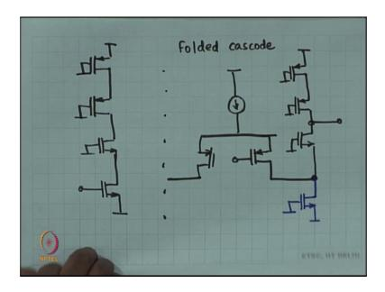
My half circuit look like this alright. Now, what if I say let us twist this and can I make this as the half circuit also? Is this also good half circuit? Of course, this is also a good half circuit, because it is exactly the same, ok. Just that I have twisted this bottom device up, right and in the small signal picture incremental picture there is no difference between nMOS and PMOS.
