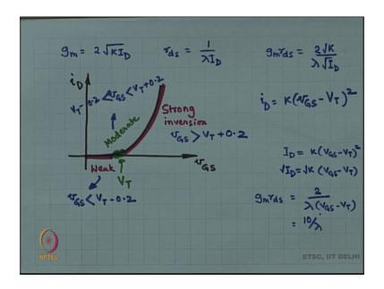
Let us do this g m is equal to two times square root of K I D r d s is 1 by lambda I D ok. The gain of the circuit best possible gain intrinsic gain of the MOSFET is g m times r d s right by the way both of these are slight approximations, but that is ok. So, this is equal to two times root K times divided by lambda divided by root I D ok. So, what this means is that, if I decrease I D, then hopefully the intrinsic gain of the MOSFET is going to increase.
