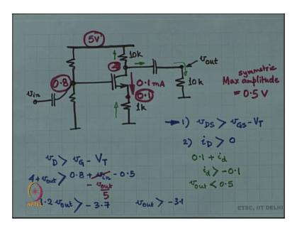
So, we had chosen 10 k over here, 10 k over here, 1 k over here, right and as far as I remember this was 5 volts, this current we had chosen was 0.1 milliamperes and, the voltage over here was 4 the voltage over here was 0.1 and the voltage at the gate was 0.8.
