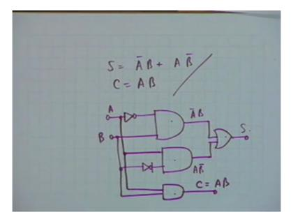
Now if I represent this half adder logic I divide the half adder logic A bar B plus AB bar I should say or A bar and B or A and B bar or I will simplify this in terms of ordinary language C is simply AB then all that I have to do is, I have to use a NOT gate for A and then I had B, had an AND gate this is A bar B. Similarly I have to have an A and B with a NOT gate another AND gate and these 2 outputs are to be ORED therefore I require another OR gate and this is S.
