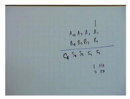
Therefore if I have let say 4 bit number to be added to another 4 bit number let say I have A4, A3, A2, A1, B1, B2, B3, B4, alright. How many half adder shall we need? Just one, half adder is required only for this, only for the first column for the others I require, how many? Obviously 3 full adder, so I require one half leather and 3 full adder, alright. The result sum 1, sum 2, sum 3, sum 4 and the carry, carry after 4.
