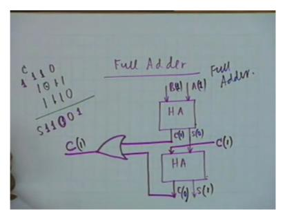
Now let us look at full adder, a full adder as I have said required to add 3 things given 2 digits, given 2 bits and the carry of the previous and therefore we shall require 2 half adder because one half adder can add only 2 bits and therefore we shall require 2 half adder, let say half adder 1 and half adder-2. Suppose I want to add let say A and B, 2 bits A and B the result would be sum and carry, it is half adder.
