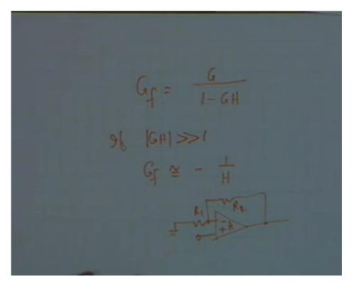
The first point was desensitising gain, alright. In order to look at that, in order to appreciate how the gain becomes insensitive in variations of the device parameters for tolerance of circuit parameters or ageing or temperature just look at this G bu 1 minus GH this is the general formula, alright. Now if GH is much greater than 1 then you seeGf becomes approximately equal to minus 1 over H.
