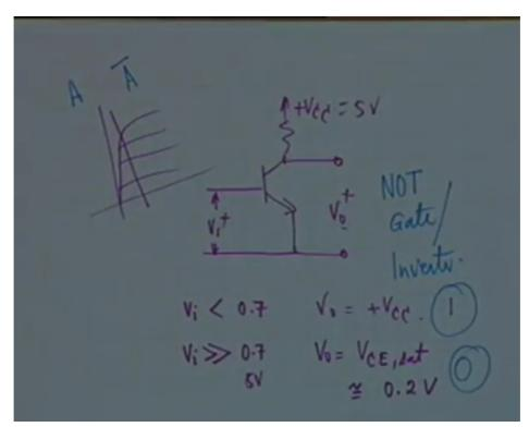
A Transistor also can act as a switch, consider a common emitter transistor plus VCC and let us say we applied input here and output is taken from here to here. If input is negative or less than 0.7 less than the threshold or the base emitter junction, if Vi is less than 0.7 then the transistor does not conduct, right? If it does not conduct then what is V0? V0 becomes equal to plus VCC.
