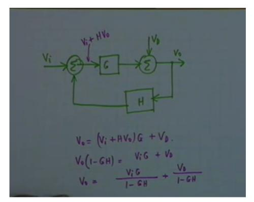
Now to this amplifier we apply now negative feedback this is V0 we apply a feedback network H and summer and this is now Vi, alright. Then V0, as you see what is this? This signal this is Vi plus H times V0, okay. And therefore V0 is equal to Vi plus HV0 multiplied by G plus VD and therefore we get V0 1 minus GH equals to ViG plus VD or V0 is equal to ViG divided by 1 minus GH plus VD divided by 1 minus GH, alright.
