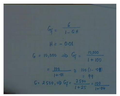
To take a more concrete illustrative example, suppose we have a feedback amplifier whose gain is G by 1 minus GH and take some specific example, let say H equal to if it is to be negative feedback then H must be negative, suppose H is minus 0.01 very small fraction of the output, 1 percent of the output is fed back to the input and suppose G is equal to let say 10,000, can you tell me what GF is?
