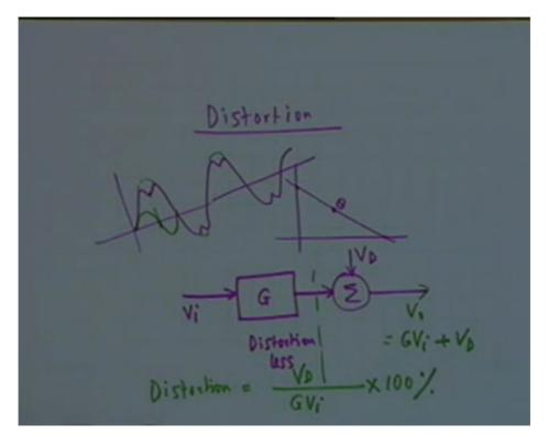
Next we look at distortion, how it reduces distortion? Distortion cannot happen in small signal amplifiers, in small signal amplifiers the signal excursion is around a small region around the Q point there is no distortion we have linear amplification but suppose we take a large signal amplifier like power amplifier where the excursion is between the extreme limit then obviously we reach non-linear region's and therefore there will be distortion.
