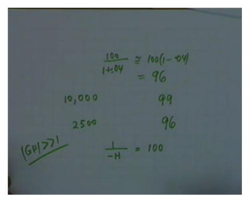
I can write this as 100, can I change the page? 100 divided by 1 plus 0.04 is approximately equal to hundred 1 minus 0.04 and you see this is only equal to 96. So gain change from 10,000 to 2500, a drop, a change by 75 percent makes a change of the feedback amplifier gain only to the extent of 3 percent 99 to 96, is that clear? 75 percent change here is reflected only as 3 percent change and therefore the gain becomes insensitive to the gain of the internal amplifier.
