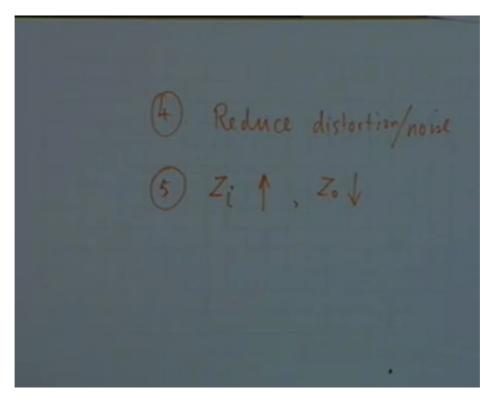
Then the 4th reason why negative feedback is used, is that negative feedback is used to reduce distortion and noise in the output of an amplifier. Negative feedback reduces distortion and the fifth reason amongst many others, fifth major reason is negative feedback helps to increase the input impedance and decrease the output impedance. We shall look at each of this separately, alright.
