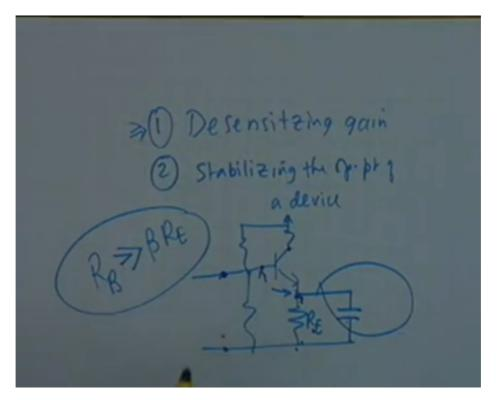
So desensitising gain then we have already studied stabilising the operating point of the device. You recall that the BJP biasing, this resistance RE or there are other resistances, this resistance RE for AC it is to be shorted, virtually shorted, why was this needed? Because otherwise the gain is reduced, why is the gain reduced? Because if this capacitor is not there then RE acts as negative feedback and this is very easy to see.
