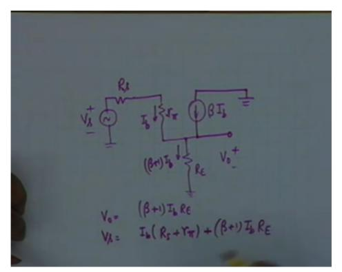
And to analyze this you draw the small signal equivalent circuit Vs then Rs then you ignore RB, R1 parallel R2 you ignore or include this in rpi where you cannot include even rpi here, why not? Because RB does not come in parallel with rpi, rpi goes to R sub E and that goes to ground alright. Then you have a current generator beta IB, if this current is IB beta IB then where does this go?
