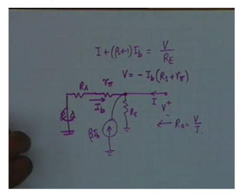
Now let us see how to calculate this? So we draw the circuit backwards we have an RE, a close RE which an actor voltage source V and we find out the current I then R0 would be equal to V by I and if I look at the circuit what I have is an rpi and an Rs the current through this is I sub B and no voltage this is shorted, the voltage source should be shorted and then we also had across RE current coming to this note from ground and therefore we have beta Ib from ground, alright.
