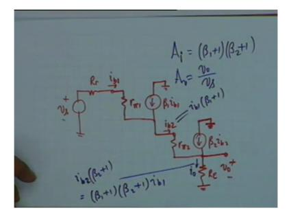
And therefore this goes to ground. Now this current whatever the current is goes to the second transistor B2 and we have rpi2. So this current is ib2 and then we have beta 2 ib2 the 2 come together, where does this go? Ground once again and then this current now flows to R sub e and this is the circuit is v0, this is the equivalent circuit and you can very easily analyze this just by looking just by commonsense.
