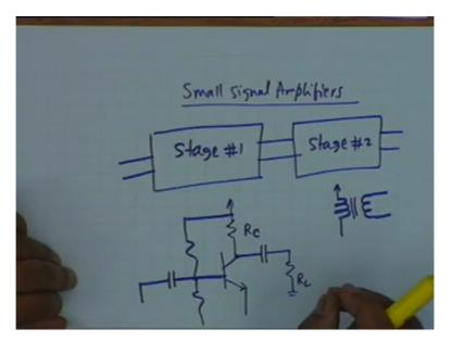
This is the model that we are now going to utilize to analyze small signal amplifiers and we shall introduce a couple of terms in this connection and then leave it for tomorrow's class. A small signal amplifier usually is classified according to the coupling that one makes from one stage to another. Stage 1 to stage 2, when 1 transistor is not enough for gaining you may have to use multiple transistors and the way stage one is connected to stage 2 is technically called coupling which is obvious.
