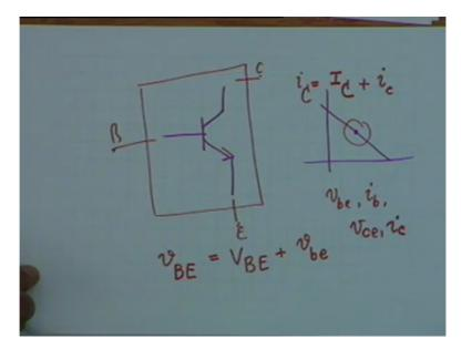
Now let us look at a transistor and for the specific lessons it a common emitter transistor while you know we have to use DC, you have to use power supply VCC, we have to use resistances to biasthe transistor properly and you know we have to determine a Q point at the middle of the load line to make maximum possible swing and all that.
