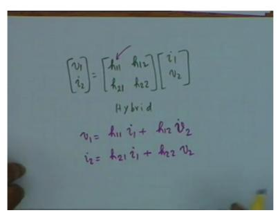
If we expand this relation, let me rewrite v1 i2 is the h parameter i1 v2 this parameters are named in the same manner that means recall h11, h12 first row first column is h11, first row second column h12, second row first column h21 and h22 and these are called hybrid parameters, hybrid, H y b r i d. You can see very clearly that h11 for example, how would you define h11? h11 is v1 divided by i1 with v2 equal to 0, alright.
