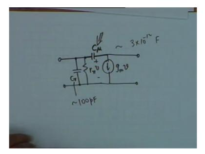
For the purpose of this course and for the rest of the lectures we shall be satisfied with a simplified model, we shall ignore rx and therefore what we will have is in an rpi, in parallel it is Cpi and this voltage is v then I shall have current generator of gmv and very unfortunate this capacitor Cmui is inferior very small capacitor of the order of 3pugs that is 3 times 10 to the minus 12 farad.
