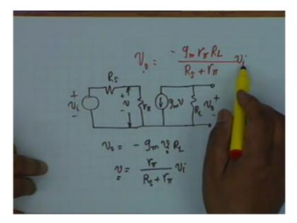
The most elementary amplifier that is we have a that is vi, perhaps we can include a source resistance Rs then of course we have the DC bias let say VBB, is the polarity correct? The base should be positive with respect to emitter, this is a PNP transistor and suppose in the collector circuit we have a load RL and the collector biasing supplier minus plus and this is VCC, this is our elementary amplifier and we want to know, what is the signal voltage across RL?
