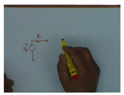
If I draw the equivalent circuit I have vs in (()) (42:53) with Rs then for Q1 I have rpi 1, alright. And I have beta 1, if this current is I sub B1 I have beta 1 ib1, where does this go? This point is the collector.
