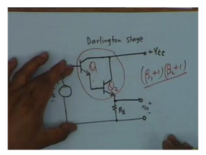
If you look at this circuit, you see this voltage minus vbe 1 minus vbe2 is this voltage and for AC this voltage should be exactly equal to the AC of this voltage which means that the voltage gain should be equal to 1.
