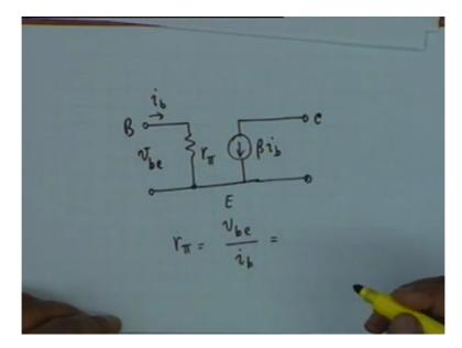
Beta ib and therefore my equivalent circuit simply becomes rpi, this is vbe, this current is i sub b and we have beta i sub b that is it. This is the collector, this is the base band this is the emitter, this is the equivalent circuit of the common emitter transistor. Well, you can find out what rpi is? rpi as I said is the dynamic resistance of the forward biased diode and therefore rpi shall be **it is** it is clear it is vbe divided by ib, alright. And you know what this is?
