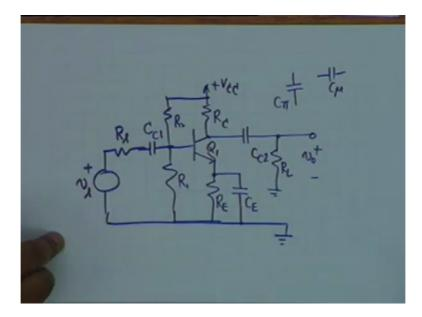
And a simple small signal amplifier that we shall analyze in great details next time is the most familiar circuit in which there is one transistor Q1, it is coupled to the load through a capacitor CRL, the base is biased to R1 and R2 this is called the self biasing circuit and the input is coupled through let us say Rs and vs our purpose will be to determine the voltage v0 in terms vs and that will determine the gain.
