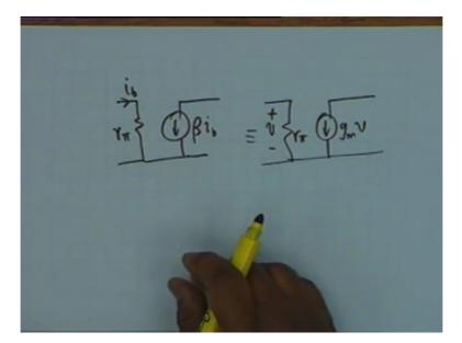
So we shall use either of these 2 circuits one is called the rpi beta circuit beta ib, this is ib equivalent second of the transistor or the same circuit represented like this, we shall use this as small v, it is vbe actually and we shall represent this as gmv this is your circuit, alright. They are absolutely equivalent to each other. Suppose now we make an amplifier, we make amplifier.
