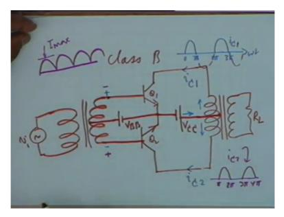
Let us look at these once more. Input power, what does the battery give out? iC1 plus iC2, now iC1 plus iC2, obviously is the full rectified sign, is not that right? And what is the DC that is drawn from the battery? The average value of this, if this is Imax then what is the average value? 2 by pi multiplied by Imax.
