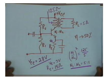
25 is given by the load line, 25 is a Q point, alright. That is this will be the VCE plus the voltage drop across the emitter resistance that means not 0.7 we are not going to (()) (8:43) which is still 25, VCC shall be able to drop in the transformer 0, the drop in the collector to emitter 25 plus 3 volts and therefore VCC shall be 28 volts, alright.
