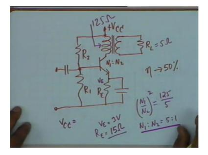
Now suppose in the transformer coupled amplifier the actual load could be as low as let us say 5 volts. Suppose this is 5 ohms, what you want here is 125 ohms and therefore N1 is to N2 whole square should be equal to 125 divided by 5 in other words N1 is to N2 should be equal to 5 is to 1 that means if the secondary has 10 turns then the primary should have 50 turns okay.
