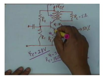
And you can calculate VBB from the requirement that VBE is 0.7, this voltage is 0.7, this is 3 volts, so this is 3.7, alright. VBB minus 3.7 shall be equal to IB times RB from which you can determine RB and therefore you can determine both R1 and R2 this calculation is routine and I shall not carry this out.
