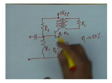
Instead of a resistance in the collector we had the transformer primary and to be secondary is connected the load, actual load RL which could be a loudspeaker and then this goes to plus VCC and usual biasing circuit there is a resistance R sub 2 and there is a resistance R sub 1 the input signal is applied between these 2 points (()) (2:07) voltage source or a current either a voltage source or a current source this is RE and this is a bypass capacitor.
