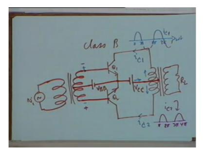
Now let us look at the typical class we operation. As I said in class B operation you use 2 transistors, okay. You use 2 transistors like this and in the base circuit you take this signal through the transformer, this is your signal to be amplified Vi, alright. And the base bias is provided by VBB like this. This VBB I have shown it schematically but it is obviously derive from VCC through a potential divide.
