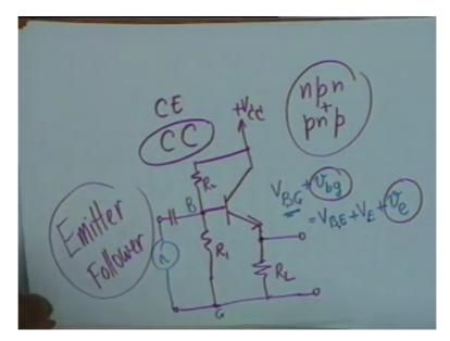
If you make a combination of NPN and PNP then you can avoid the transformer. Let me draw this circuit first then I will explain. The circuit the circuit uses what is known as, we have known common emitter amplifier, circuit uses common collector stages that is each of these stages NPN and PNP stage which are connected in a push pull configuration they are instead of CE the CC that means the collector is common between input and output.
