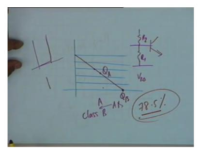
Now suppose you go to the other extreme that is you take a transistor let us look at the base side base circuit only. Suppose instead of a positive battery here, instead of positive VDD you connected negative VBB, alright. Then you see if you are applying A through a capacitor, if you are applying an input signal here which varies like this, alright. Then transistor will conduct only when Vi exits VBB, is not that right? By at least 0.7 volts otherwise the transistor will not conduct.
