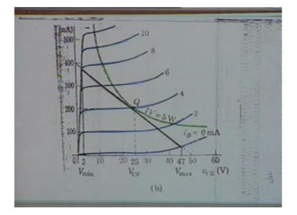
Now if we go back to this operation to this transistor characteristic once more, you notice that if we choose our Q point here then for the input current, what is the input current? The base current, the base current is 4 milliampere, now suppose the base current the AC input is such that the base current varies from let us say 2 milliampere to 6 milliampere.
