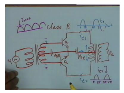
If you look at the circuit again is there any drop here in the transformer, no. And therefore VCC must be the Q point, agree? The load line must we, the DC load line is a vertical load line, agree? Is this point clear VCC is equal to V-max? No, it is not clear, alright.
