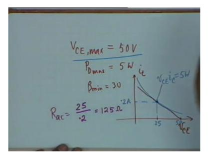
Illustrate the design of a transformer coupled amplifier, we take a typical example in which the same specifications for the transistor hole as was used in the previous example of transformer less power amplifier that is resistance load. Suppose we have a transistor in which the maximum VCE is 50 volts, the maximum power dissipation is 5 watt let us say beta min is equal to 30 the same specifications we have used in the previous example.
