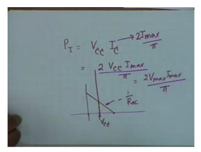
You recall this in the characteristics if this is the AC load line then the middle point is the Q point. This represents minus 1 by Rac this is the Q point, alright. Now what is this? What is the relation between this point and VCC? This must be the VCC because the DC resistance of the transformer primary is 0 and therefore the DC load line must be vertical wherever the DC load line cuts is VCC, alright.
