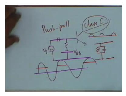
And class C the efficiency can go further up, it can go to as much as 85 percent or so, alright. 85 percent, now the problem of distortion as you see in class B operation, as I said 2 transistors are used one takes care of positive half cycle the other of the negative of cycle and the 2 outputs are so combined that a full-cycle of the output is obtained, so there is no distortion.
