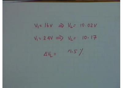
For example, suppose V1 is 16 volts. This gives you VL equal to, I have calculated this to 10.02 volt. If V1 now increases, the DC voltage increases by 50 percent which means that V1 equal to 24 volt, from 16 to 24 is 50 percent increase, then VL changes only to 10.17. You seehow constant it remains for a while and fluctuation here from 16 to 24, the load voltage changes only from 10.02 to 10.17. And Delta VL if you calculate this, 0.15, oh it issimply how much? 1.5 percent. That is it.
