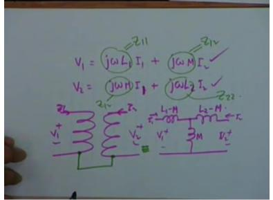
Now suppose I write J omega L1 as Z11, J omega M as Z12, is as Z12 and this as Z22, then do not you see that this is simply the same T model, that is Z11 minus Z12, Z22 minus Z12 and this is simply Z12. Is that okay? So instead of looking at it from the impedance parameters, OC impedance parameters, we look at it directly in terms of the components. Well, there are 2 things that one should notice.
