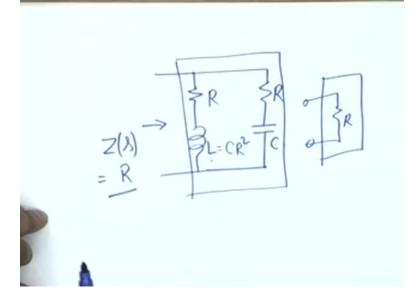
It is the problem that we had talked about in one of the classes when the lights went off. It is a complicated resonant circuit. It is a parallel resonant circuit in which L and C are in parallel but unfortunately both of them have a series resistance of capital R and in addition, the elements are so conspired that L becomes L is equal to CR square. You can see that the impedance if you calculate in terms of S, it is simply R. We had discussed this?
