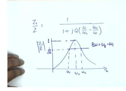
And therefore we get a universal form of expression for the dimensionless ratio of impedances. This is 1 by 1 + JQ. From both of these terms, I can take Q outand then I write omega by omega 0 - omega 0 by omega. All right? I can do that. Now obviously, this will have a maximum when omega by omega 0 equals to omega 0 by omega. That means, when omega equal to omega 0, the maximum value is 1. This is independent of the actual values of resistance, inductance and capacitor.
