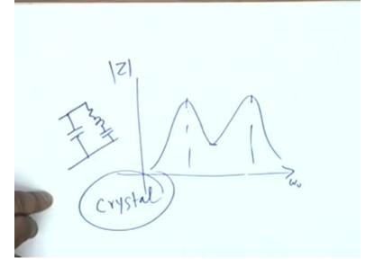
For example, we can have circuits like this. All right? Resonating at 2 different frequencies. This is also resonance. A minimum in the characteristic is also resonance. For example, it could be the plot of the impedance vs frequency. If it is the plot of the impedance vs frequency, then what will you call these 2 frequencies? The impedance is a maximum, these 2 must be corresponding to parallel or series? That is the question I am asking.
