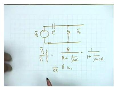
It does not take very long to show that the circuit containing a capacitor and a resistance what kind of circuit is this? It is also a high pass filter and I can write down the ratio of V 0 to V i as equal to yes R divided by R + 1 over j Omega C and this can be written as 1 divided by 1 + 1 over j Omega C R and if I write 1 by C R, 1 by C R is the dimension of frequency.
