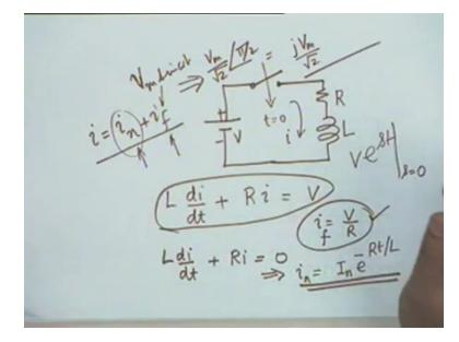
For example here I argue that the impedance of the inductor shall be 0 because s equal to 0 and that helped us determine this V the response the forced response. On the other hand if this
