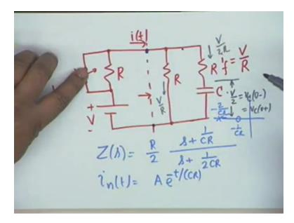
Therefore, the total current i t shall be equal to V by R + A e to the power – t divided by C R. The question now is, how do I determine the constant A? Obviously, I shall have to take i of 0 into account, the initial condition however what is the initial condition?
