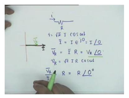
So in the case of the resistor if we go back, if we wish to draw a diagram that is the currents or voltages then you see the current is in this direction let us say this represents the current phasor I then the voltage phasor is in phase with the current phasor that is the voltage phasor also has an angle 0 to the voltage phasor maybe up to this on different scales, current and voltage cannot be represented on the same scale for this would be V R phasor.
